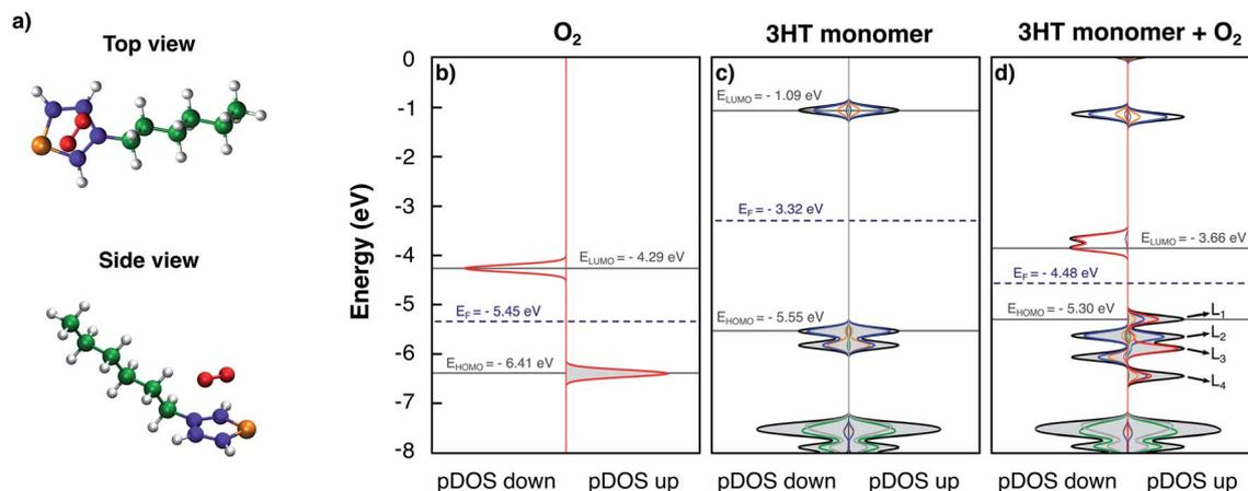
Fig. 1 Top and side view of the equilibrium geometry of the 3HT:O<sub>2</sub> system shown in a). DOS and pDOS of an isolated O<sub>2</sub> molecule b), an isolated 3HT-monomer c) and the 3HT:O<sub>2</sub> system d). Colours refer to the atoms as they are colour coded in a): oxygen – red, sulphur – orange, thiophene carbon – blue, alkyl carbon – green, and hydrogen – grey. Occupied states are indicated by grey shading.
