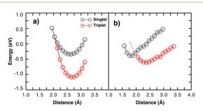
Fig. 5 Single point energy calculation for two different thiophene sites (3 and 4) of a twisted 13-3HT oligomer. The energy—distance profile of the two sites exhibits two different types: Type 1, shown in a); and Type 2, in b). Red dashed-line is the extrapolated points for d < 2.0 Å.
