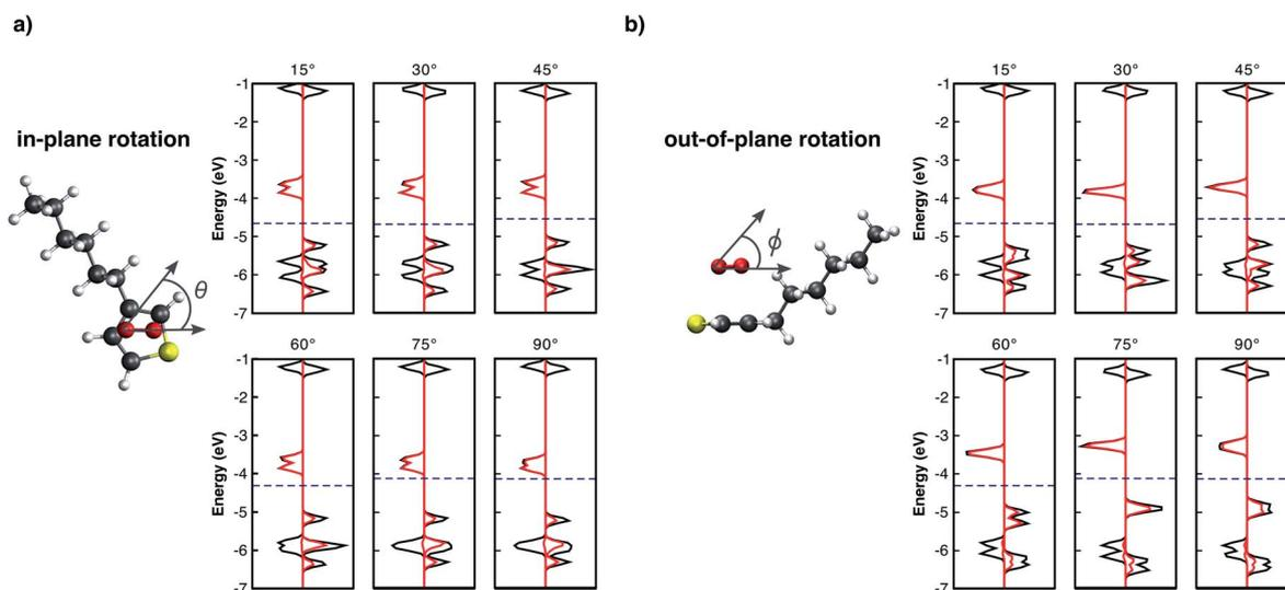
Fig. 3 DOS (black lines) of the 3HT:O<sub>2</sub> system, as well as the pDOS (red lines) of oxygen molecule, for different single point calculations. Fermi levels are displayed by the blue dashed-lines. a) Shows the in-plane angle rotation  $\theta$ , and b) the out-of-plane angle  $\phi$ .
