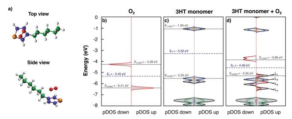
Fig. 1 Top and side view of the equilibrium geometry of the  $3HT:O_2$  system shown in a). DOS and pDOS of an isolated  $O_2$  molecule b), an isolated 3HT-monomer c) and the  $3HT:O_2$  system d). Colours refer to the atoms as they are colour coded in a): oxygen – red, sulphur – orange, thiophene carbon – blue, alkyl carbon – green, and hydrogen – grey. Occupied states are indicated by grey shading.
