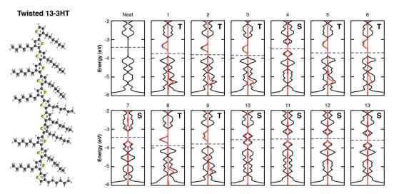
Fig. 4 Electronic structure of the neat twisted 13-3HT (first), as well as the 13-3HT: $O_2$  complex, in which each band structure corresponds to the site position of the  $O_2$  molecule with respect to the thiophene ring number (top-to-bottom).
