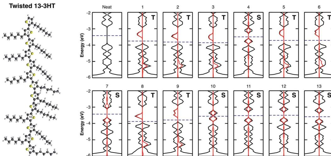
Fig. 4 Electronic structure of the neat twisted 13-3HT (first), as well as the 13-3HT:O<sub>2</sub> complex, in which each band structure corresponds to the site position of the O<sub>2</sub> molecule with respect to the thiophene ring number (top-to-bottom).
