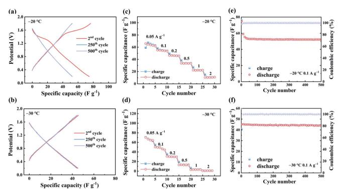
Fig. 3 Low-temperature electrochemical performance of ZHSCs using ferrocene/AC cathode. GCD curves at 0.1 A g $^{-1}$ : (a) -20 °C; (b) -30 °C; rate performance with various current densities ranging from 0.05-2 A g $^{-1}$ : (c) -20 °C; (d) -30 °C; long-term cycling at 0.1 A g $^{-1}$ : (e) -20 °C; (f) -30 °C.
