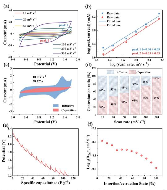
Fig. 2 Electrochemical kinetic studies of ZHSCs using ferrocene/AC cathode. (a) CV curves; (b) fitting plot between log(i) and log(v); (c) capacitive contribution to the total stored charge from CV analysis at 10 mV s<sup>-1</sup> (the red region); (d) the capacitive and diffusion contribution ratios to the total capacity at different scan rates; (e) discharge curve in GITT measurements; (f)  $Zn^{2+}$  diffusion coefficient during the discharge process.
