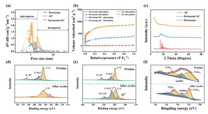
Fig. 5 (a) Pore size distribution curve; (b) N<sub>2</sub> adsorption/desorption isotherms; (c) XRD patterns of AC, ferrocene and ferrocene/AC; XPS images of (d) C 1s spectrum of AC cathode; (e) C 1s spectrum of ferrocene/AC cathode; (f) Fe 2p spectrum of ferrocene/AC cathode.
