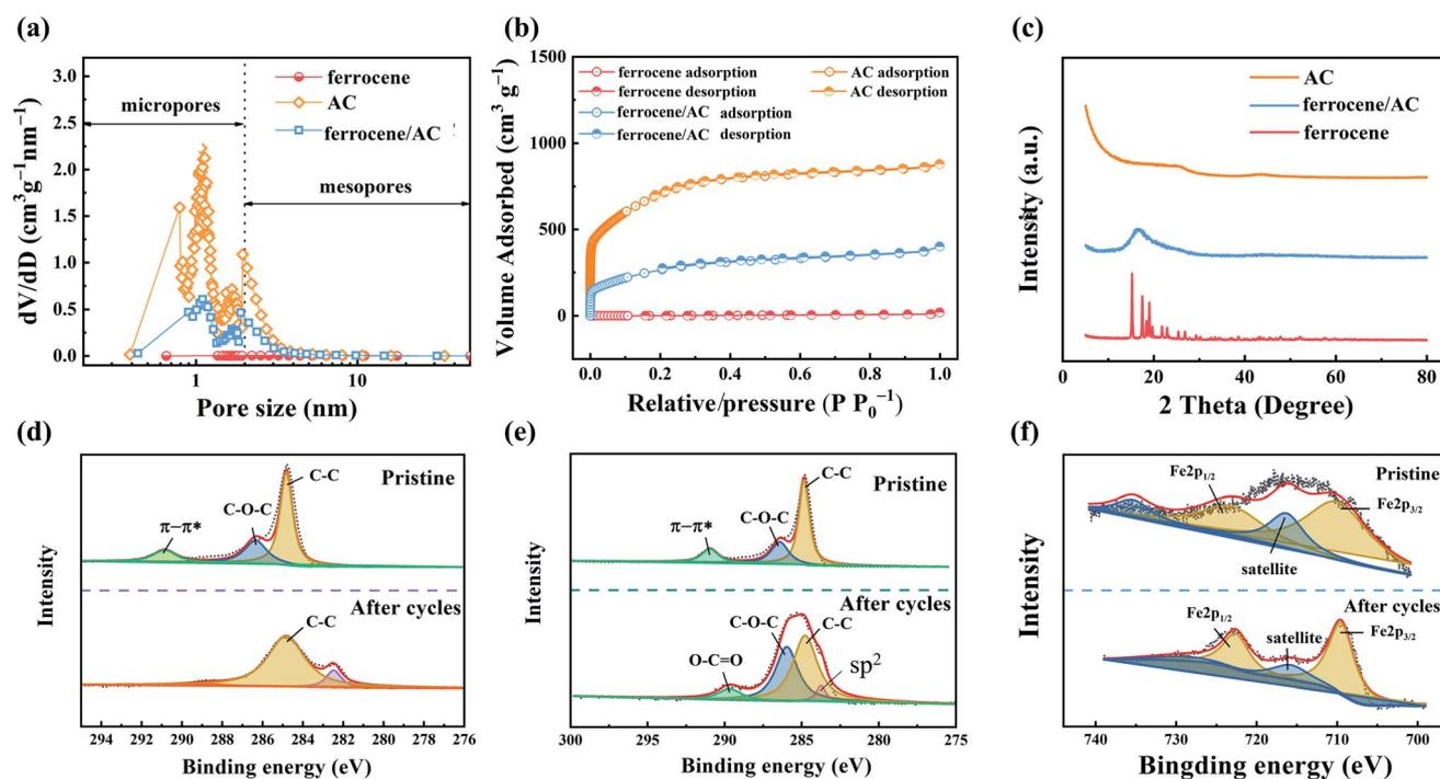
Fig. 5 (a) Pore size distribution curve; (b)  $N_2$  adsorption/desorption isotherms; (c) XRD patterns of AC, ferrocene and ferrocene/AC; XPS images of (d) C 1s spectrum of AC cathode; (e) C 1s spectrum of ferrocene/AC cathode; (f) Fe 2p spectrum of ferrocene/AC cathode.
