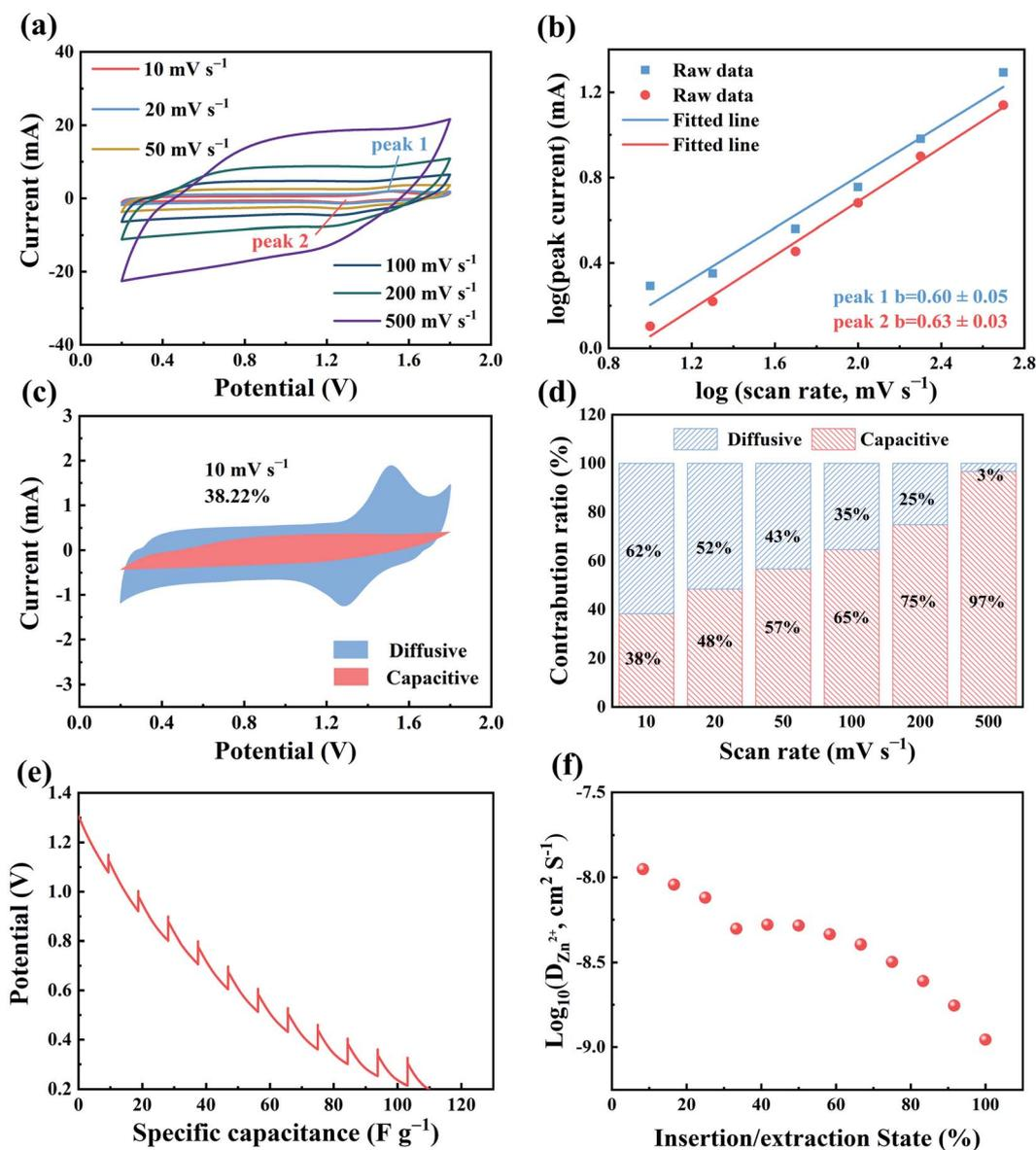
Fig. 2 Electrochemical kinetic studies of ZHSCs using ferrocene/AC cathode. (a) CV curves; (b) fitting plot between  $\log(i)$  and  $\log(v)$ ; (c) capacitive contribution to the total stored charge from CV analysis at 10 mV s<sup>-1</sup> (the red region); (d) the capacitive and diffusion contribution ratios to the total capacity at different scan rates; (e) discharge curve in GITT measurements; (f) Zn<sup>2+</sup> diffusion coefficient during the discharge process.
