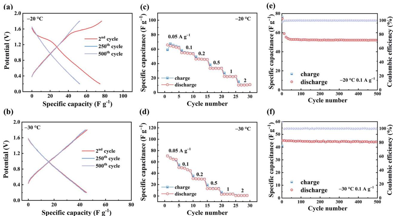
Fig. 3 Low-temperature electrochemical performance of ZHSCs using ferrocene/AC cathode. GCD curves at  $0.1 \text{ A g}^{-1}$ : (a)  $-20 \text{ }^\circ\text{C}$ ; (b)  $-30 \text{ }^\circ\text{C}$ ; rate performance with various current densities ranging from  $0.05$ – $2 \text{ A g}^{-1}$ : (c)  $-20 \text{ }^\circ\text{C}$ ; (d)  $-30 \text{ }^\circ\text{C}$ ; long-term cycling at  $0.1 \text{ A g}^{-1}$ : (e)  $-20 \text{ }^\circ\text{C}$ ; (f)  $-30 \text{ }^\circ\text{C}$ .
