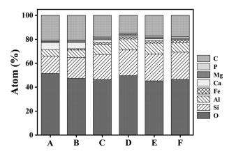
Fig. 7 Variation of atomic fraction of soil element by EDS along the soil chronosequence.
