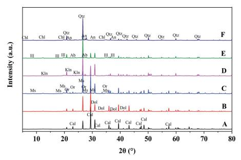
Fig. 9 X-ray diffractogram patterns (Cu K $\alpha$  radiation) and mineral change of soil aggregates along the soil chronosequence (Cal = calcite; Chl = chlorite; Dol = dolomite; Ill = illite; Kln = kaolinite; Ms = muscovite; Or = orthoclase; Qtz = quartz; An = anorthite; Ab = albite).
