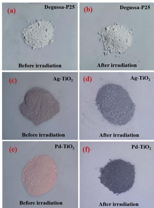
Fig. 10 (a)–(f) represent the photochromic effect in Degussa-P25, Ag<sup>+</sup> doped TiO<sub>2</sub>, and Pd<sup>2+</sup> doped TiO<sub>2</sub>, respectively.
