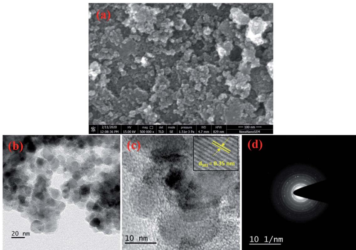
Fig. 3 (a) SEM micrographs, (b) bright field TEM image, (c) HR-TEM with interplanar  $d$ -spacing, and (d) SAED pattern of Ag-TiO<sub>2</sub>.
