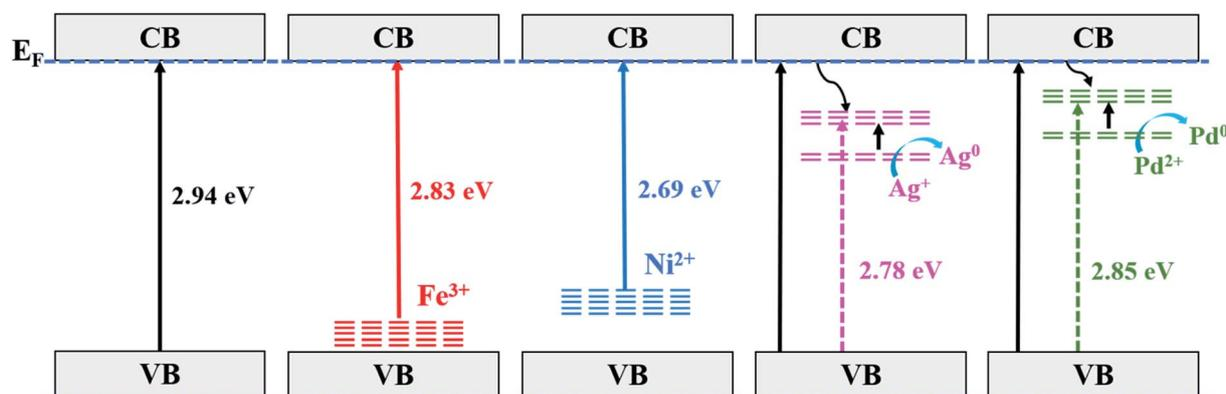
Fig. 9 A schematic representation of the different energy levels of  $\text{Ti}_{1-x}\text{M}_x\text{O}_{2-\delta}$  (M = Fe, Ni, Ag, and Pd;  $x = 0, 0.01$ ).
