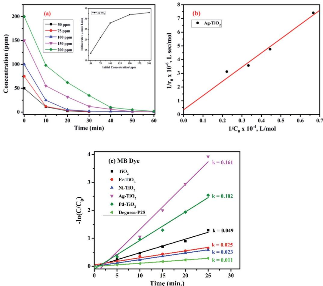
Fig. 8 (a) The effect of initial dye concentration on the degradation rate of MB with  $\text{Ag-TiO}_2$  and (b) the Langmuir–Hinshelwood plot for MB dye with  $\text{Ag-TiO}_2$ . (c) A comparison of the degradation kinetics of all the combustion synthesized photocatalysts using MB dye.
