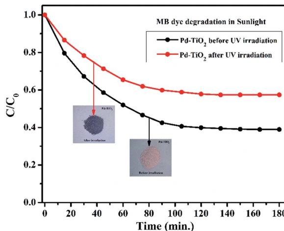
Fig. 11 Degradation of MB dye in sunlight using Pd<sup>2+</sup> doped TiO<sub>2</sub> samples before and after UV irradiation.
