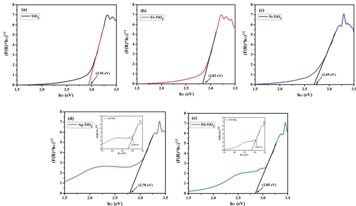
Fig. 5 (a)–(e) Kubelka–Munk plot of  $\text{Ti}_{1-x}\text{M}_x\text{O}_{2-\delta}$  ( $\text{M} = \text{Fe}, \text{Ni}, \text{Ag}, \text{and Pd}; x = 0, 0.01$ ). Insets of (d) and (e) represent the baseline approach for band gap estimation of  $\text{Ag}^+$  and  $\text{Pd}^{2+}$  doped  $\text{TiO}_2$ .
