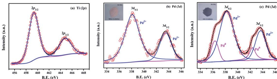
Fig. 4 (a) Ti (2p) core level spectra, and (b) and (c) Pd (3d) core level spectra of Pd<sup>2+</sup> doped TiO<sub>2</sub> before and after UV irradiation, respectively.
