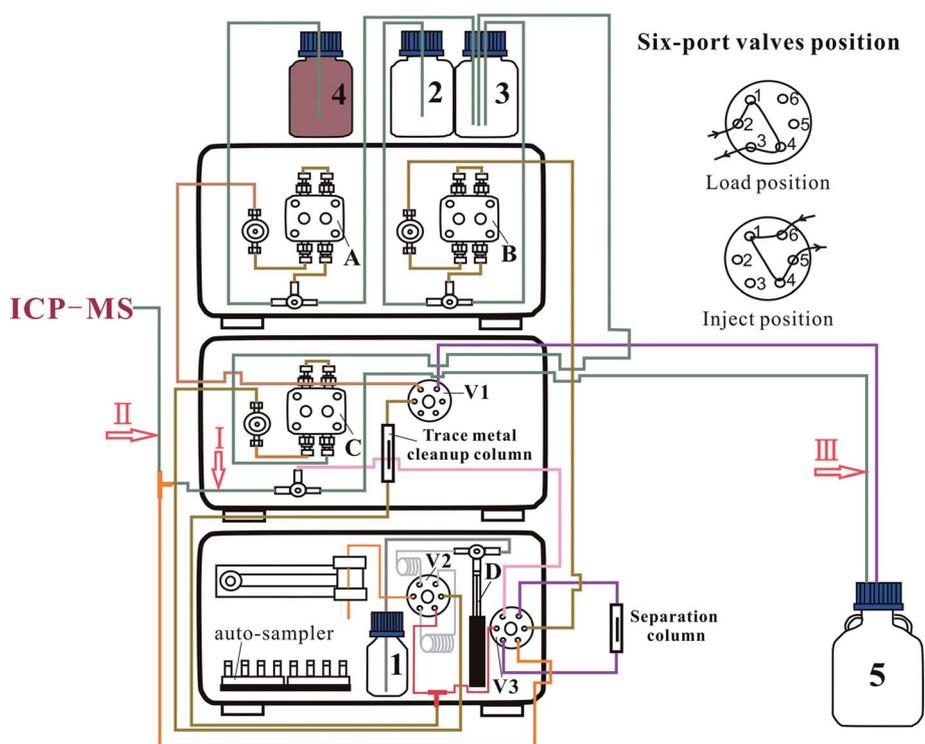
Fig. 1 Schematic configuration of the ELSPE-2 Precon system. 1 and 3: deionized water; 2: 5%  $\text{HNO}_3$ ; 4: ammonium acetate buffer; 5: waste; I and II: PTEE pipes with inner diameters of  $\geq 0.25$  mm; III: polytetrafluoroethylene pipe with a 0.5 mm inner diameter; A: ammonium acetate pump; B:  $\text{HNO}_3$  pump; C: water pump; D: syringe pump; V1, V2, and V3: six-port valves.
