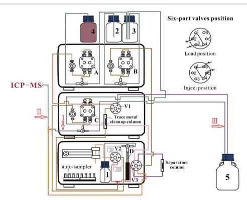
Fig. 1 Schematic configuration of the ELSPE-2 Precon system. 1 and 3: deionized water; 2: 5% HNO<sub>3</sub>; 4: ammonium acetate buffer; 5: waste; I and II: PTEE pipes with inner diameters of  $\geq$ 0.25 mm; III: polytetrafluoroethylene pipe with a 0.5 mm inner diameter; A: ammonium acetate pump; B: HNO<sub>3</sub> pump; C: water pump; D: syringe pump; V1, V2, and V3: six-port valves.
