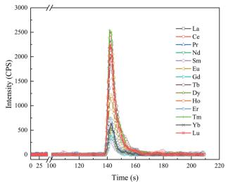
Fig. 2 Typical chromatograms of the REEs in a mixed REE standard solution (5 ng L<sup>-1</sup>), as obtained using the ELSPE-2 Precon automated separation system and online ICP-MS.
