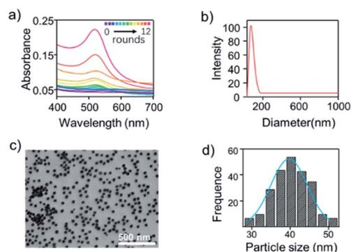
Fig. 2 Characterization of AuNPs after 12 rounds of seed growth. (a) UV-vis spectra of gold colloids from 12 different growth processes. (b) Dynamic light scattering map of AuNPs. (c) TEM image of AuNPs,  $n = 200$ . (d) Particle size distribution histogram of AuNPs from (c).
