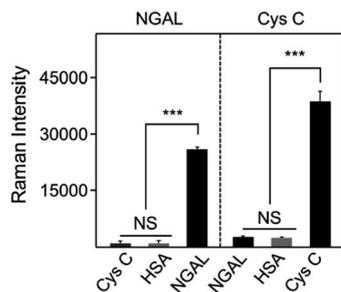
**Fig. 5** Selectivity of aptasensor for NGAL and Cys C. Raman intensity at  $1618\text{ cm}^{-1}$  of the NGAL (Cys C) aptasensor for the detection of Cys C, HSA, and NGAL (NGAL, HSA, and Cys C) with the concentration of  $200\text{ }\mu\text{g mL}^{-1}$ . Each group of experiments was tested in parallel three times.
