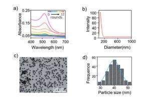
Fig. 2 Characterization of AuNPs after 12 rounds of seed growth. (a) UV-vis spectra of gold colloids from 12 different growth processes. (b) Dynamic light scattering map of AuNPs. (c) TEM image of AuNPs, n =200. (d) Particle size distribution histogram of AuNPs from (c).
