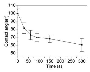
Fig. 7 Contact angle of diluted microcapsule sample M5 on the surface of cabbage leaves.
