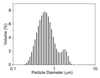
Fig. 5 Particle size distribution of microcapsule sample M5.
