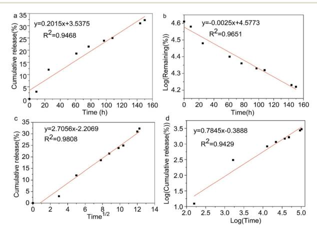
Fig. 11 Kinetic plots of chlorfenapyr microcapsule: (a) zero-order equations; (b) first-order equations; (c) Higuchi equations; (d) Korsmeyer–Peppas equations.
