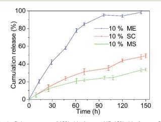
Fig. 9 Release curves of 10% chlorfenapyr ME, 10% chlorfenapyr SC and 10% chlorfenapyr MS.
