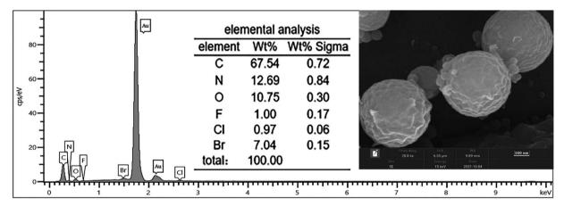
Fig. 4 SEM/EDS image of microcapsule.
