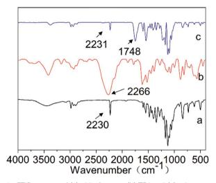
Fig. 6 FTIR spectra of (a) chlorfenapyr, (b) TDI and (c) microcapsule sample M5.
