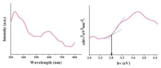
Fig. 4 UV-DR spectra of the Co-C<sub>3</sub>N<sub>4</sub>-Imine/TiO<sub>2</sub> nanohybrid.
