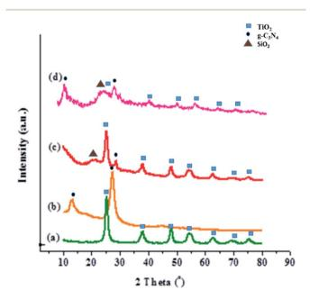
Fig. 3 XRD pattern of (a) TiO<sub>2</sub>, (b)  $g-C_3N_4$ , (c)  $g-C_3N_4$ -imine/TiO<sub>2</sub>, and (d) the Co- $g-C_3N_4$ /TiO<sub>2</sub> nanohybrid.
