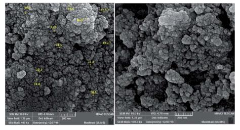
Fig. 2 SEM images of the Co-g-C<sub>3</sub>N<sub>4</sub>-imine/TiO<sub>2</sub> nanohybrid
