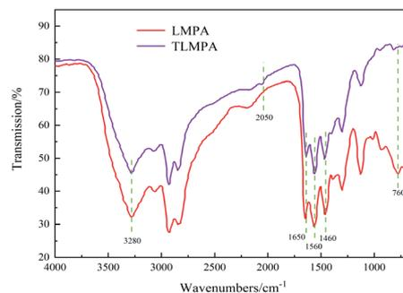
Fig. 4 FTIR diagram of thiourea modified hardener.
