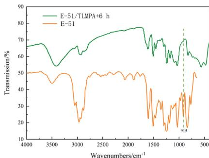
Fig. 5 FTIR diagram after curing at 25 °C for 6 h.
