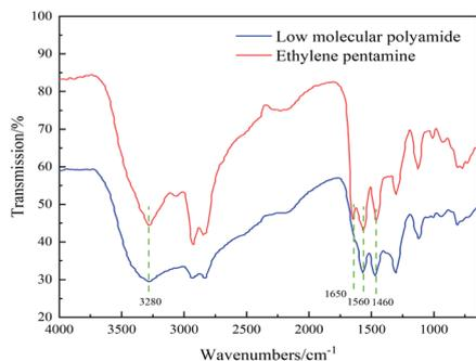
Fig. 3 FTIR diagram of ethylene pentaamine and low molecular polyamide.
