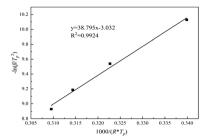
Fig. 7 Linear fitting of  $ln(\beta/T_p^2)$  and  $1/(R \times T_p)$  modified hardener.
