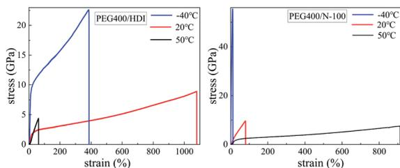
Fig. 17 The stress–strain curves of NEPE binder systems.
