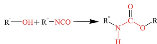
Fig. 2 Curing reaction mechanism.
