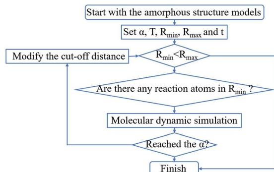
Fig. 3 Flow chart of the crosslinking reaction algorithm.
