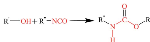
Fig. 2 Curing reaction mechanism.
