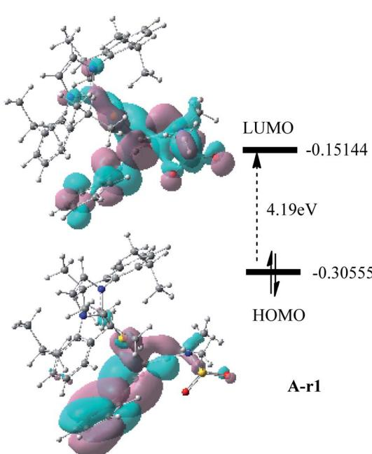
Fig. 1 Frontier molecular orbitals and orbital energies of A-r1.
