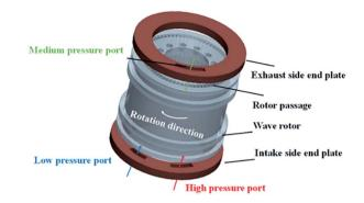
Fig. 1 A schematic diagram of the fundamental components of a gas wave ejector.
