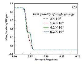
Fig. 7 Grid independence verification: (a) a comparison of pressure distributions; (b) a comparison of component distributions
