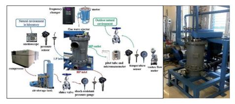
Fig. 17 A schematic diagram of the components and procedure used for the GWE experimental system with a photograph of the set up.
