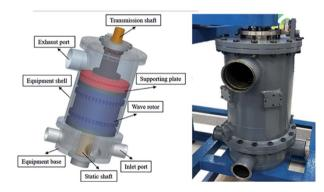
Fig. 18 The experimental GWE equipment.
