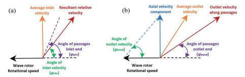
Fig. 8 Schematic diagrams of the gas incident and exhaust angles: (a) gas incident angle  $\varphi_{\text{vin}}$ : (b) gas exhaust angle  $\varphi_{\text{vout}}$
