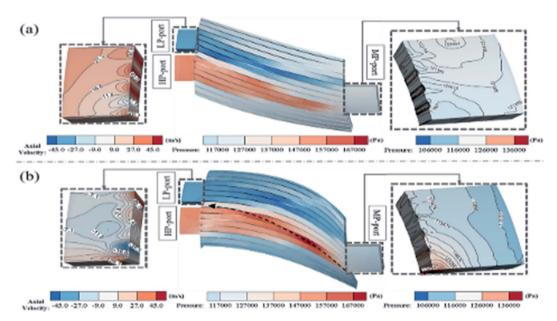
Fig. 11 Contour maps of state parameter distributions in the models: (a) the model with  $\varphi_{pin}=60^{\circ}$  and  $\varphi_{pout}=75^{\circ}$ ; (b) the model with  $\varphi_{pin}=90^{\circ}$  and  $\varphi_{pout}=30^{\circ}$ .
