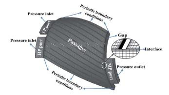
Fig. 6 Schematic diagram of numerical calculation model and meshing.
