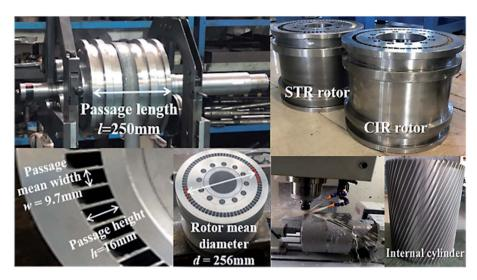
Fig. 19 Photographs showing the wave rotor parameters used in the experiments.
