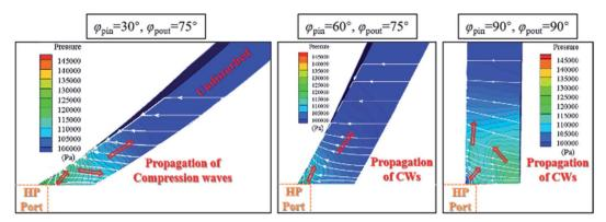
Fig. 13 A comparison of pressure distributions in channels with  $t_{\text{open}}/t_{\text{po}} = 0.2$  (the white arrow lines depict streamlines).
