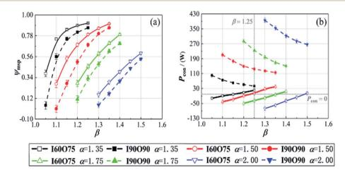
Fig. 22 The experimental results regarding (a) the static pressure increase ratio  $\psi_{\rm msp}$  and (b) the gas loading power consumption  $P_{\rm con}$
