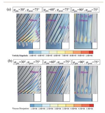
Fig. 16 A comparison of parameter distributions in the channels: (a) vorticity intensity (values below  $2\times 10^{-5}$  are not shown); and (b) viscous dissipation (values below  $10^{-6}$  are not shown).
