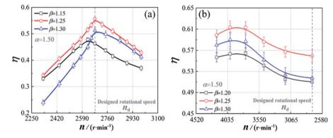
Fig. 23 The variations in the I60O75 rotor efficiency  $\eta$  with rotor rotation speed: (a) fixed pressure ports; (b) pressure ports satisfying optimal matching.
