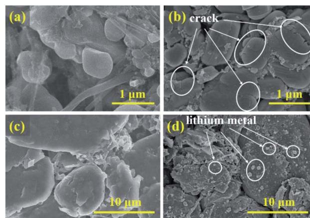
Fig. 7 SEM images of the positive electrode of (a) the new battery and (b) after 500 cycles at  $-10\text{ }^{\circ}\text{C}$ ; SEM images of the negative electrode of (c) the new battery and (d) after 500 cycles at  $-10\text{ }^{\circ}\text{C}$ .
