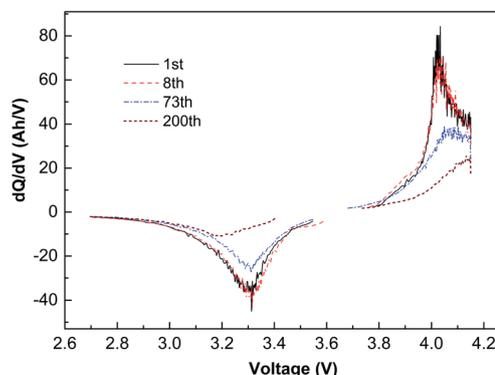
Fig. 4 Capacity differential curves cycling with 1C at -10, and voltage 2.7–4.15 V.
