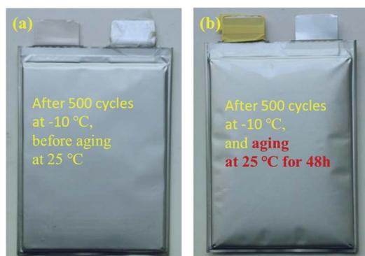
Fig. 6 (a) Photograph of the battery after 500 cycles at  $-10\text{ }^{\circ}\text{C}$ ; (b) photograph of the battery stored for 48 h at  $25\text{ }^{\circ}\text{C}$  after  $-10\text{ }^{\circ}\text{C}$  cycling.
