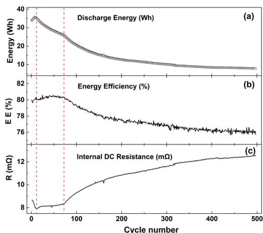
Fig. 5 The curves of (a) discharge energy, (b) discharge energy efficiency and (c) full state DC internal resistance with cycle times at  $-10\text{ }^{\circ}\text{C}$  at a current of 1C current over a voltage range of 2.7–4.15 V.
