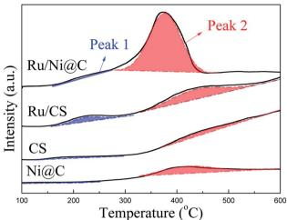
Fig. 7 NH<sub>3</sub>-TPD profiles of catalysts.
