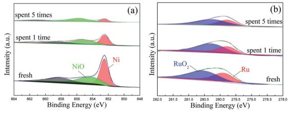
Fig. 11 XPS spectra of fresh and spent Ru/Ni@C. (a) Ni  $2p_{2/3}$ , (b) Ru  $3d_{5/3}$ .
