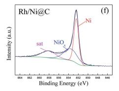
Fig. 5 Ni 2p<sub>3/2</sub> XPS spectra of various M/Ni@C catalysts.
