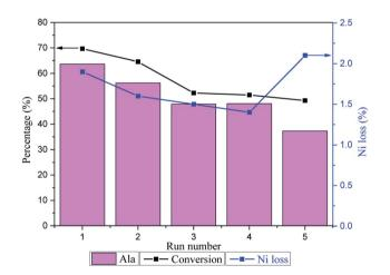
Fig. 9 Recycle test of the Ru/NiaC catalyst and the Ni loss in the reaction solution. Reaction conditions: LA 0.1 g, NH $_3$ ·H $_2$ O (28 wt%) 10 mL, 473 K, H $_2$  1.5 MPa, 2 h.
