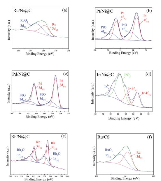
Fig. 6 M metal XPS spectra of various M/Ni@C catalysts.
