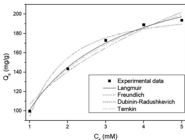
Fig. 7 Non-linear adsorption isotherm models for strontium by ST2 at different concentration at equilibrium.
