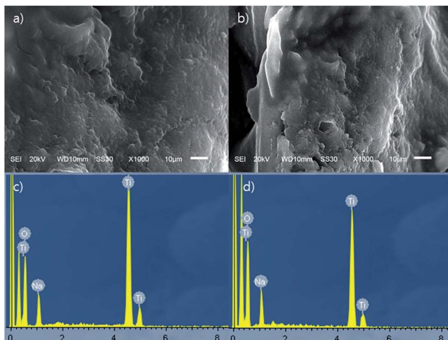
Fig. 1 SEM pictures and EDS profile data of ST1 and ST2; (a) SEM picture of ST1, (b) SEM picture of ST2, (c) EDS profile of ST1, and (d) EDS profile of ST2.
