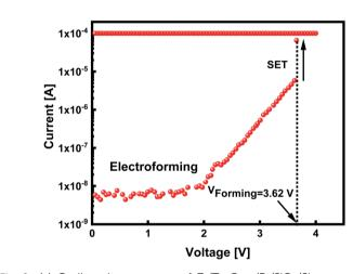
Fig. 2 (a) Cyclic voltammogram of Zr/Ta $_2$ O $_{5-x}$ /Pt/SiO $_2$ /Si memory device. (b) The typical forming curve of Zr/Ta $_2$ O $_{5-x}$ /Pt/SiO $_2$ /Si device with a sudden current transition where the device turns in the ON state. Current compliance of 100  $\mu$ A was imposed to avoid the complete breakdown of the device.
