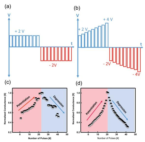
Fig. 6 Various programming pulse schemes. (a) Successive identical and (b) non-identical neuron spikes. (c and d) Normalized potentiation and depression properties of  $TaO_{2-x}$  thin-film memristor with two different pulse schemes. The non-identical spikes lead to a linear synaptic behavior with a slope of 1. Using nonidentical presynaptic spikes, a significant improvement in symmetry was observed.
