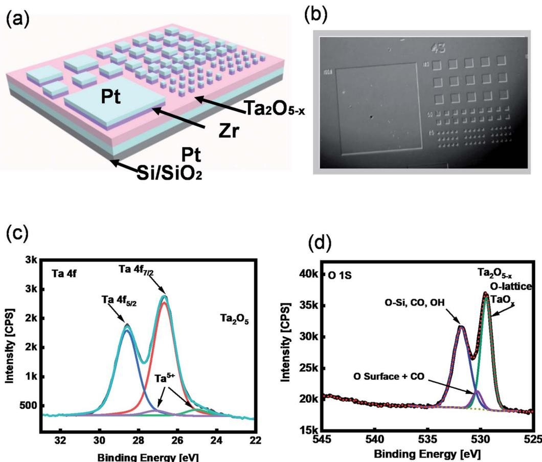
Fig. 1 (a) Schematic illustration of the ECM memory device with  $\text{Ta}_2\text{O}_{5-x}$  solid electrolyte (SE) and  $\text{Zr}/\text{Ta}_2\text{O}_{5-x}/\text{Pt}/\text{SiO}_2/\text{Si}$  structure; the ECMs are with various dimensions ( $2\ \mu\text{m}$  to  $500\ \mu\text{m}$ ). (b) Optical image of the devices fabricated by photolithography. (c) XPS core level of Ta 4f and (d) O 1s.
