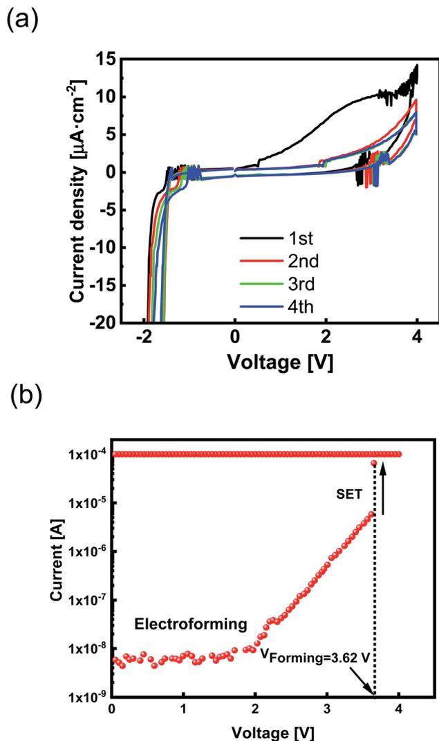
Fig. 2 (a) Cyclic voltammogram of Zr/Ta<sub>2</sub>O<sub>5-x</sub>/Pt/SiO<sub>2</sub>/Si memory device. (b) The typical forming curve of Zr/Ta<sub>2</sub>O<sub>5-x</sub>/Pt/SiO<sub>2</sub>/Si device with a sudden current transition where the device turns in the ON state. Current compliance of 100 μA was imposed to avoid the complete breakdown of the device.
