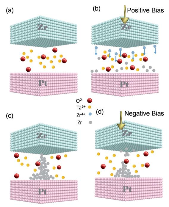
Fig. 4 (a) Proposed operation mechanism of the electro metallization cell. (a) Pristine state. (b) Set process;  $Zr^{4+}$  ions are reduced to  $Zr^{0}$  at the top electrode; ion movement under positive bias voltage; (b) reducing of Zr cations which provide a source for filament formation. (c) The Zr-based conductive filament is formed and causes a connection between two electrodes. (d) OFF state; Zr filament ruptures in the solid electrolyte under negative bias.
