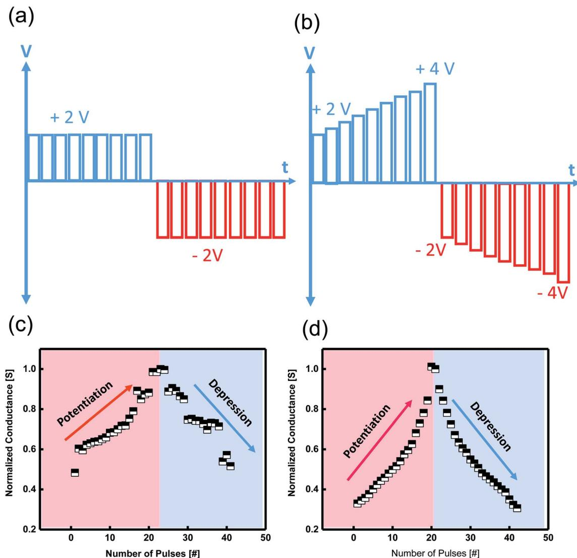
Fig. 6 Various programming pulse schemes. (a) Successive identical and (b) non-identical neuron spikes. (c and d) Normalized potentiation and depression properties of TaO<sub>2-x</sub> thin-film memristor with two different pulse schemes. The non-identical spikes lead to a linear synaptic behavior with a slope of 1. Using nonidentical presynaptic spikes, a significant improvement in symmetry was observed.
