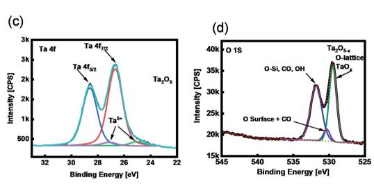
Fig. 1 (a) Schematic illustration of the ECM memory device with  $Ta_2O_{5-x}$  solid electrolyte (SE) and  $Zr/Ta_2O_{5-x}/Pt/SiO_2/Si$  structure; the ECMs are with various dimensions (2  $\mu$ m to 500  $\mu$ m). (b) Optical image of the devices fabricated by photolithography. (c) XPS core level of Ta 4f and (d) O 1s.
