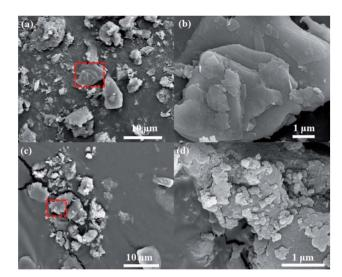
Fig. 2 SEM images in different sizes of bulk g-C $_3$ N $_4$ : 10  $\mu$ m (a) and 1  $\mu$ m (b), g-C $_3$ N $_4$ -¹BuONa: 10  $\mu$ m (c) and 1  $\mu$ m (d).
