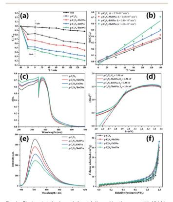
Fig. 4 Photocatalytic degradation (a), linear kinetic curves (b), UV-Vis DRS (c), corresponding bandgaps (d), PL spectra (e), and  $N_2$  adsorption–desorption isotherms (f) of bulk g-C<sub>3</sub>N<sub>4</sub>, g-C<sub>3</sub>N<sub>4</sub>–MeONa, g-C<sub>3</sub>N<sub>4</sub>–EtONa, and g-C<sub>3</sub>N<sub>4</sub>– $^t$ BuONa.
