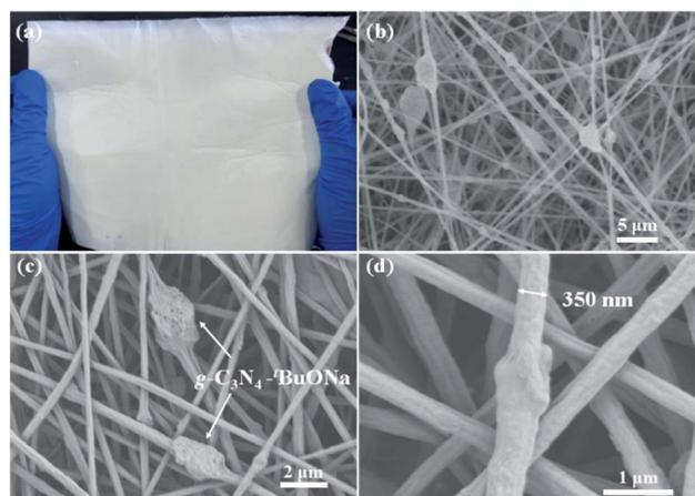
Fig. 5 (a) Paper-based floating photocatalyst PAN/ $g\text{-C}_3\text{N}_4\text{-}^t\text{BuONa}$  (A4 size, 210 mm  $\times$  297 mm) and SEM images for comparison: 5  $\mu\text{m}$  (b), 2  $\mu\text{m}$  (c) and 1  $\mu\text{m}$  (d).
