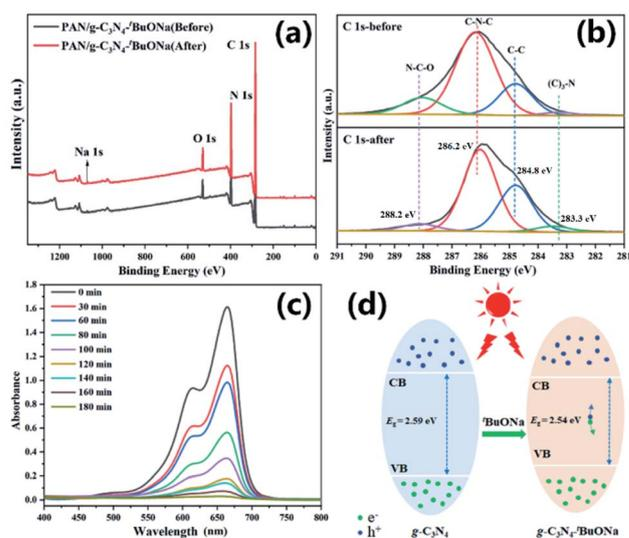
Fig. 7 (a) XPS full-spectra and (b) C 1s core-level spectra of PAN/ $g\text{-C}_3\text{N}_4\text{-tBuONa}$  before and after cyclic degradation, (c) the alteration of UV-Vis absorption profile from 0 to 180 minutes, (d) schematic bandgap diagrams from  $g\text{-C}_3\text{N}_4$  to  $g\text{-C}_3\text{N}_4\text{-tBuONa}$ .
