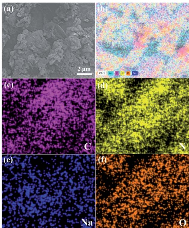
Fig. 3 (a) SEM image of g-C<sub>3</sub>N<sub>4</sub>-<sup>t</sup>BuONa and (b–f) mapping images of the total, C, N, Na, and O elements, respectively.
