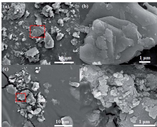
Fig. 2 SEM images in different sizes of bulk g-C<sub>3</sub>N<sub>4</sub>: 10 μm (a) and 1 μm (b), g-C<sub>3</sub>N<sub>4</sub>-<sup>t</sup>BuONa: 10 μm (c) and 1 μm (d).
