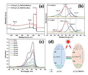
Fig. 7 (a) XPS full-spectra and (b) C 1s core-level spectra of PAN/g- $C_3N_4-^tBuONa$  before and after cyclic degradation, (c) the alternation of UV-Vis absorption profile from 0 to 180 minutes, (d) schematic bandgap diagrams from g- $C_3N_4$  to g- $C_3N_4-^tBuONa$ .
