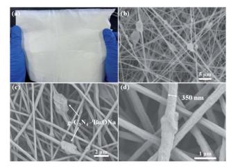
Fig. 5 (a) Paper-based floating photocatalyst PAN/g-C<sub>3</sub>N<sub>4</sub>-<sup>t</sup>BuONa (A4 size, 210 mm  $\times$  297 mm) and SEM images for comparison: 5  $\mu$ m (b), 2 μm (c) and 1 μm (d).
