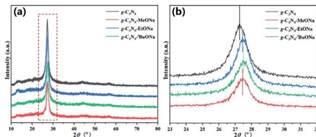
**Fig. 1** (a) XRD patterns of the bulk  $g-C_3N_4$ ,  $g-C_3N_4$ -MeONa,  $g-C_3N_4$ -EtONa, and  $g-C_3N_4$ - $t$ BuONa powders; (b) (002) magnified image of XRD patterns.
