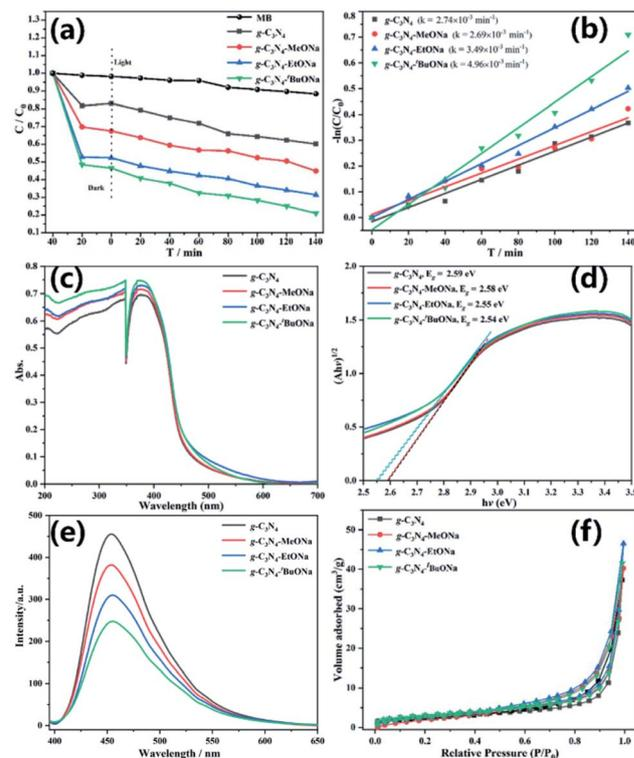
Fig. 4 Photocatalytic degradation (a), linear kinetic curves (b), UV-Vis DRS (c), corresponding bandgaps (d), PL spectra (e), and N<sub>2</sub> adsorption-desorption isotherms (f) of bulk g-C<sub>3</sub>N<sub>4</sub>, g-C<sub>3</sub>N<sub>4</sub>-MeONa, g-C<sub>3</sub>N<sub>4</sub>-EtONa, and g-C<sub>3</sub>N<sub>4</sub>-<sup>t</sup>BuONa.
