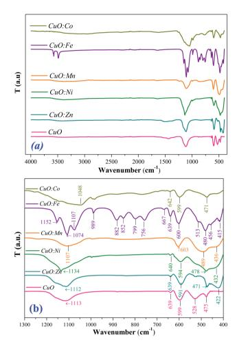
Fig. 5 FTIR spectra of CuO and TM-doped CuO NPs (a) in 400–4000  $\rm cm^{-1}$  range, and (b) enlarged spectra from 400  $\rm cm^{-1}$  to 1300  $\rm cm^{-1}$ .
