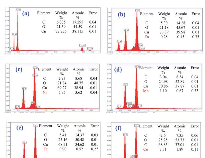
Fig. 7 EDX spectra of (a) undoped CuO, (b) CuO:Zn, (c) CuO:Ni, (d) CuO:Mn, (e) CuO:Fe, and (f) CuO:Co NPs.
