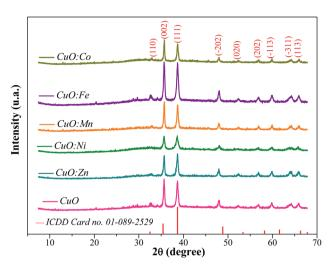
Fig. 1 XRD patterns of CuO, CuO:Fe, CuO:Mn, CuO:Co, CuO:Zn and CuO:Ni samples.
