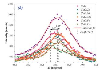
Fig. 2 The Gaussian fit to the (a) (002) and (b) (111) diffraction peaks of undoped and TM-doped CuO NPs.
