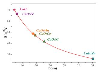
**Fig. 4** Relationship between the SSA and the average crystallite size (*D*) of undoped and TM-doped CuO NPs.
