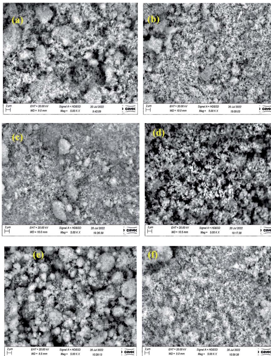
Fig. 6 High magnification SEM images of (a) undoped CuO, (b) CuO:Zn, (c) CuO:Ni, (d) CuO:Co, (e) CuO:Fe, and (f) CuO:Mn.
