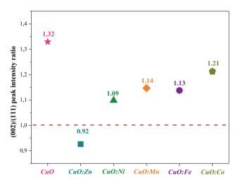
Fig. 3  $I_{(002)}/I_{(111)}$  peak intensity ratio of undoped and TM-doped CuO NPs.
