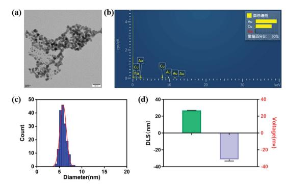
Fig. 1 (a) TEM, (b) EDS, (c) particle size distribution, (d) size and ζ-potential of core-shell Cu/Au NPs. Error bars represent the standard deviation of three repeated measurements.
