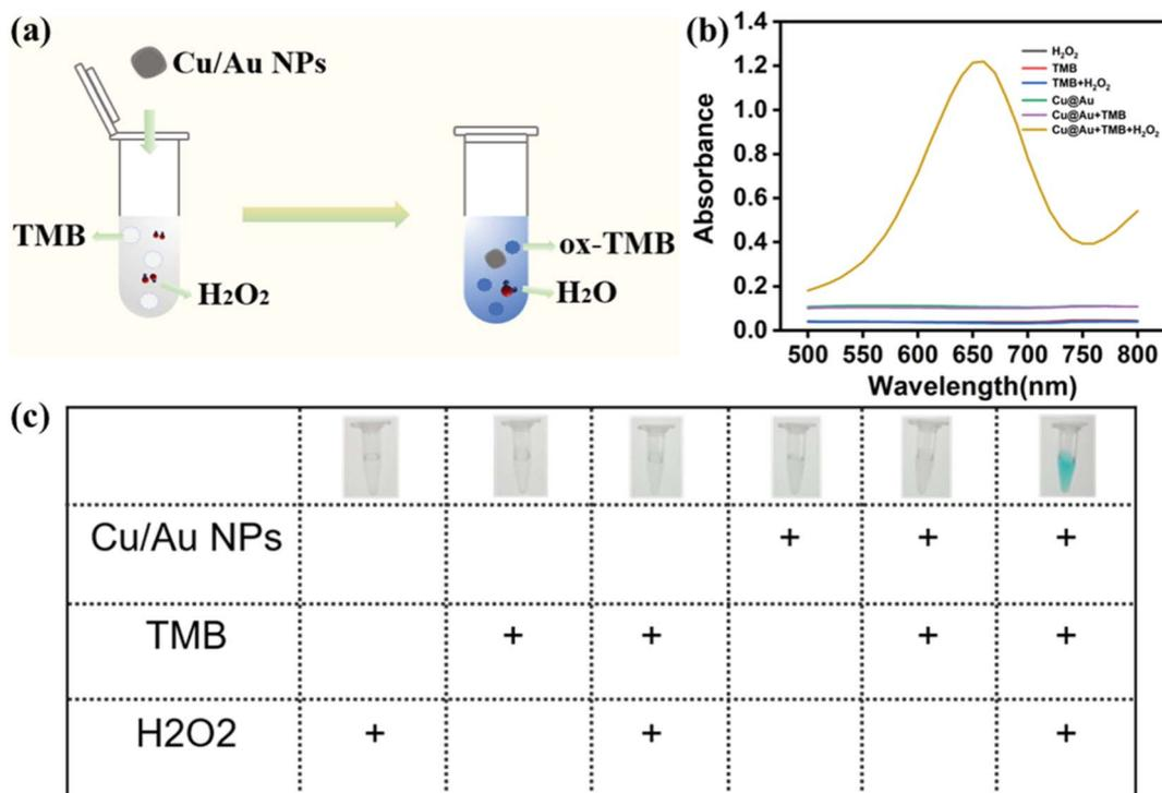
Fig. 3 (a) Schematic of the enzyme-like performance of core-shell Cu/Au NPs. (b) UV-vis absorbance spectrum of the core-shell Cu/Au NPs, TMB and H<sub>2</sub>O<sub>2</sub> reaction solutions and controls. (c) Visual photographs of varied control systems.
