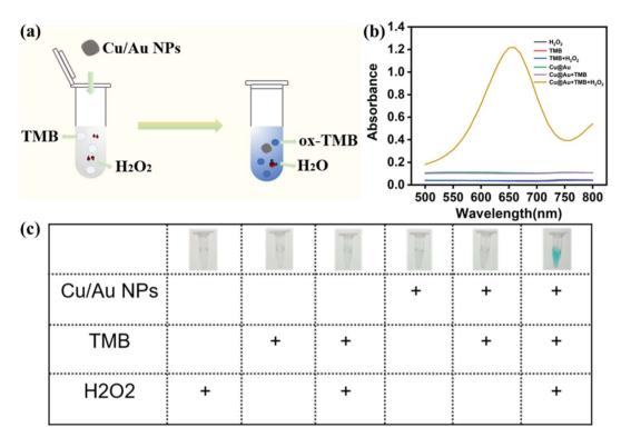
Fig. 3 (a) Schematic of the enzyme-like performance of core-shell Cu/Au NPs. (b) UV-vis absorbance spectrum of the core-shell Cu/Au NPs, TMB and H<sub>2</sub>O<sub>2</sub> reaction solutions and controls. (c) Visual photographs of varied control systems.
