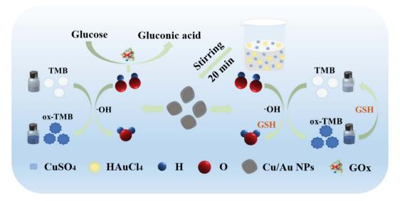
$\textbf{Scheme 1} \quad \textbf{Illustration of the preparation process for core-shell Cu/Au NPs and sensing assay $H_2O_2$, glucose and GSH. } \\$
