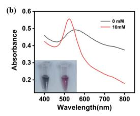
Fig. 2 (a) UV-vis absorption spectra of the solution in presence of iodide with different concentrations (0–10 mM); (b) photos and UV-vis absorption spectra of the solution containing 0/10 mM iodide, respectively (Inset: Color changes of core–shell Cu/Au NPs with 0 mM and 10 mM KI).
