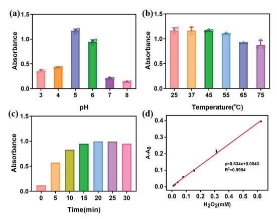
Fig. 5 Optimization of variable experimental factors of colorimetric detection; (a) pH; (b) reaction temperature; (c) reaction time; (d) the linear range of  $H_2O_2$  colorimetric detection. Error bars represent the standard deviation of three repeated measurements.
