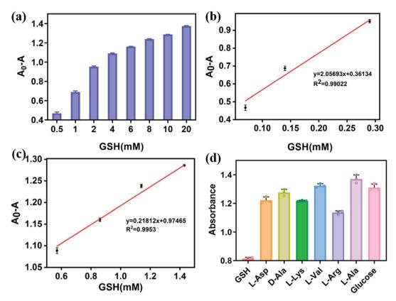
Fig. 8 (a) Linear calibration plot for GSH from 0.5 mM to 10 mM. (b) The dependence of the absorbance on the concentration of GSH in the range from 0.07 to 0.29 mM (b) and 0.57 to 1.43 mM (c). (d) Selectivity test for GSH detection by the proposed assay. GSH was 2 mM, the other amino acids were 10 mM
