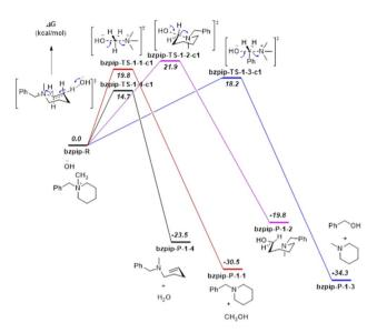
Fig. 4 DFT calculation results for the proposed reaction pathways of [Bzpip]<sup>+</sup>. Relative solvated Gibbs free energies are shown in italic bold, unit: kcal mol<sup>-1</sup>. Calculated at the B3LYP/6 6-311++G(2d,p) level with the PCM solvation model (solvent = water).
