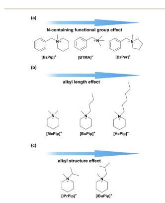
Fig. 1 Molecular designs for the optimization of alkaline stable cations for AEMs: (a) modulation of the N-containing functional group; (b) and (c) modulation of the alkyl substituent.
