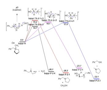
Fig. 5 DFT calculation results for the proposed reaction pathways of  $[Bzpyr]^+$ . Relative solvated Gibbs free energies are shown in italic bold, unit: kcal  $mol^{-1}$ . Calculated at the B3LYP/6 6-311++G(2d,p) level with the PCM solvation model (solvent = water).
