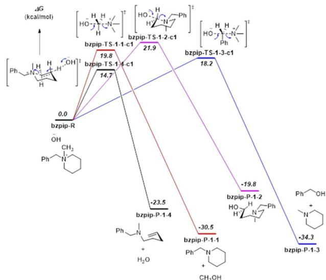
Fig. 4 DFT calculation results for the proposed reaction pathways of [Bzpip]<sup>+</sup>. Relative solvated Gibbs free energies are shown in italic bold, unit: kcal mol<sup>-1</sup>. Calculated at the B3LYP/6-311+G(2d,p) level with the PCM solvation model (solvent = water).
