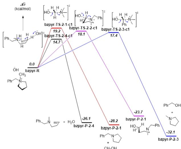
Fig. 5 DFT calculation results for the proposed reaction pathways of [Bzpyr]<sup>+</sup>. Relative solvated Gibbs free energies are shown in italic bold, unit: kcal mol<sup>-1</sup>. Calculated at the B3LYP/6-311++G(2d,p) level with the PCM solvation model (solvent = water).
