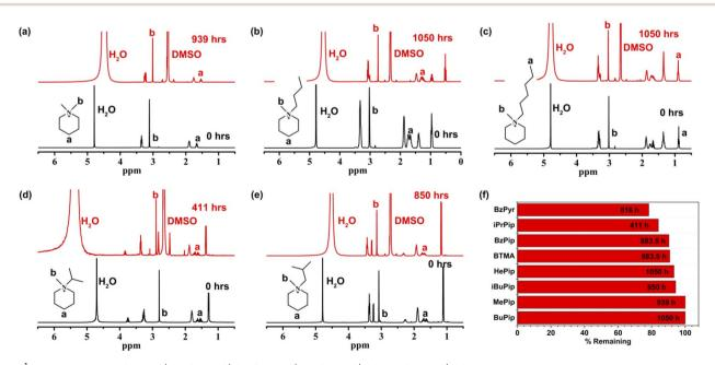
Fig. 6 <sup>1</sup>H NMR spectra of [MePip]<sup>+</sup> (a), [BuPip]<sup>+</sup> (b), [HePip]<sup>+</sup> (c), [iPrPip]<sup>+</sup> (d) and [iBuPip]<sup>+</sup> (e) before and after immersion in 7 M KOH solution at 100 °C and the remnants of these cations after the test (f).
