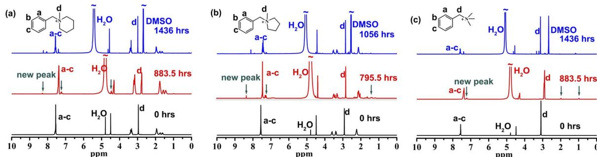
Fig. 2  $^1\text{H}$  NMR of  $[\text{BzPip}]^+$  (a),  $[\text{BzPyr}]^+$  (b) and  $[\text{BTMA}]^+$  (c) before and after immersion in 7 M KOH solution at 100 °C.
