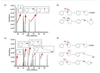
Fig. 3 GC-MS analysis of possible byproducts and potential degradation routes for [BzPip]<sup>+</sup> (a and b) and [BzPyr]<sup>+</sup> in 7 M KOH at 100 °C (c and d).
