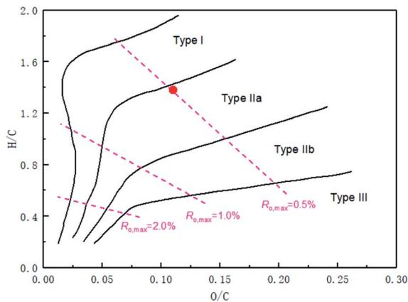
Fig. 1 Kerogen-type paradigm diagram of Tissot and Welte.
