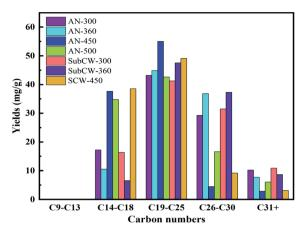
Fig. 9 Carbon number distribution of residual oil in two pyrolysis modes.
