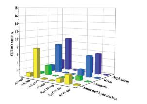
Fig. 8 Components of residual oil in anhydrous pyrolysis and sub/supercritical water pyrolysis.
