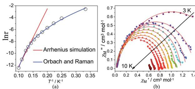
Fig. 5 Plots of relaxation time ( $\ln \tau$ ) vs.  $T^{-1}$  at applied dc fields of 2000 Oe (a). The red and blue lines are fitted with the Arrhenius law and multiple relaxation processes, respectively. Cole–Cole plots under 2000 Oe for **1** (b). The solid lines are the best fit to the experimental data.
