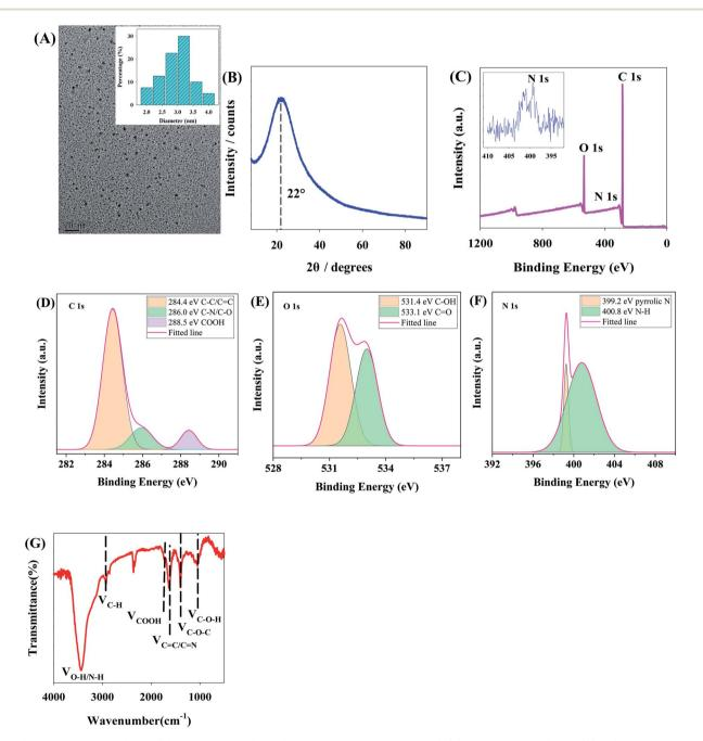
Fig. 2 Characterization of CNDs: (A) TEM image of CNDs (inset: particle size distribution); (B) XRD pattern of CNDs; (C) XPS spectrum of CNDs; (D) C 1s, (E) O 1s and (F) N 1s high-resolution spectra; (G) infrared spectrum of CNDs.
