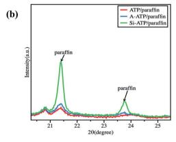
Fig. 7 (a) XRD diagrams of the pure paraffin and FSPCMs; (b) Comparison of paraffin crystallization peaks in FSPCMs ( $2\theta$  rang from  $20-25^{\circ}$ ).
