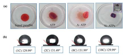
Fig. 3 (a) Observation of ATP, A-ATP and Si-ATPs absorbed the liquid paraffin (dyed with red oil for easy observation) in water; (b) the interfacial hydrophobic contact angles of Si-ATPs.
