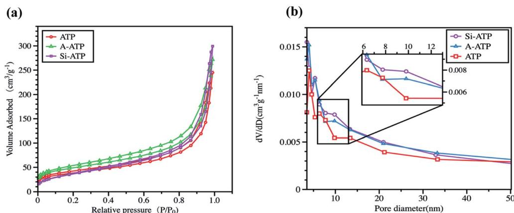
**Fig. 5** Nitrogen adsorption–desorption and pore size distribution curves of the three porous materials: (a) nitrogen adsorption–desorption isotherms, and (b) pore size distributions.
