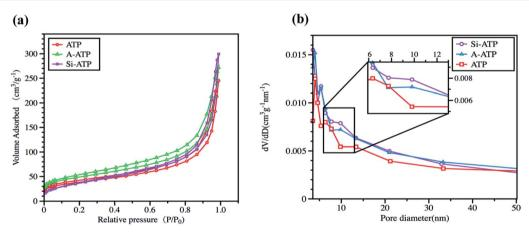
Fig. 5 Nitrogen adsorption—desorption and pore size distribution curves of the three porous materials: (a) nitrogen adsorption—desorption isotherms, and (b) pore size distributions.
