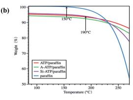
Fig. 9 (a) TGA curves of the pure paraffin and FSPCMs; (b) a part of curves from temperature range of 100–250 °C
