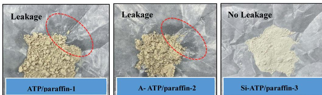
**Fig. 6** Comparison of shape-stabilized ability of the three porous materials for paraffin ( $m_{\text{porous material}} : m_{\text{paraffin}} = 5 : 3$ , 1.0 g supporting material and 0.6 g paraffin for each case).
