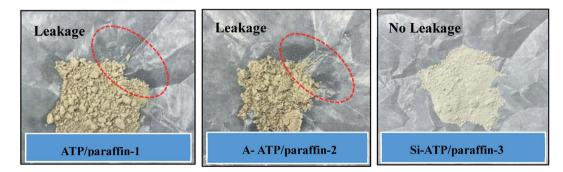
Fig. 6 Comparison of shape-stabilized ability of the three porous materials for paraffin ( $m_{porous\ material}$ :  $m_{paraffin} = 5:3,1.0$  g supporting material and 0.6 g paraffin for each case).
