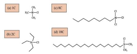
Fig. 1 Chemical structures of these chlorosilane modification reagents: (a) trimethylchlorosilane (1C); (b)triethylchlorosilane (2C); (c) n-octyltrichlorosilane (8C); (d) dimethyl octadecyl chlorosilane (18C).
