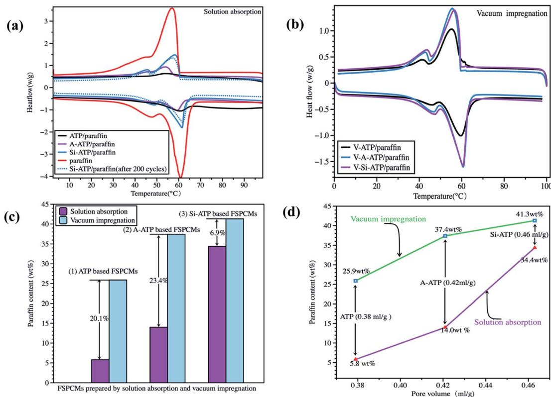
Fig. 8 (a) DSC curves of the FSPCMs prepared by solution absorption; (b) DSC curves of the FSPCMs prepared by vacuum impregnation; (c) a comparison of the FSPCMs prepared by solution absorption and vacuum impregnation; (d) paraffin content in the FSPCMs supported by porous materials with different pore volumes.
