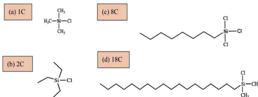
Fig. 1 Chemical structures of these chlorosilane modification reagents: (a) trimethylchlorosilane (1C); (b) triethylchlorosilane (2C); (c) *n*-octyltrichlorosilane (8C); (d) dimethyl octadecyl chlorosilane (18C).
