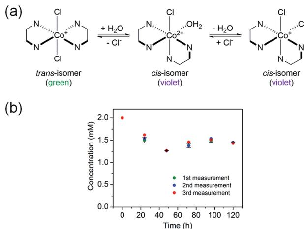
Fig. 2 (a) The *trans*–*cis* isomerization process of *trans*-[Co(en)<sub>2</sub>Cl<sub>2</sub>]<sup>+</sup> via aquation in water. (b) Time courses of the encapsulation of *trans*-[Co(en)<sub>2</sub>Cl<sub>2</sub>]<sup>+</sup> ion by as-prepared InBTB in ethanol. The measurements were performed in triplicate.
