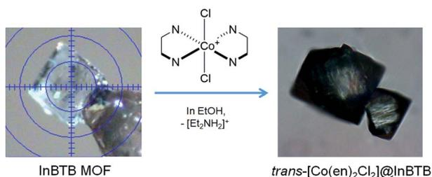
Fig. 1 Schematic of the preparation of  $\text{trans}[\text{Co}(\text{en})_2\text{Cl}_2]\text{Cl}$  into  $\text{trans}[\text{Co}(\text{en})_2\text{Cl}_2]\text{Cl}$  through the cation-exchange of  $[\text{Et}_2\text{NH}_2]^+$  with  $\text{trans}[\text{Co}(\text{en})_2\text{Cl}_2]^+$ .
