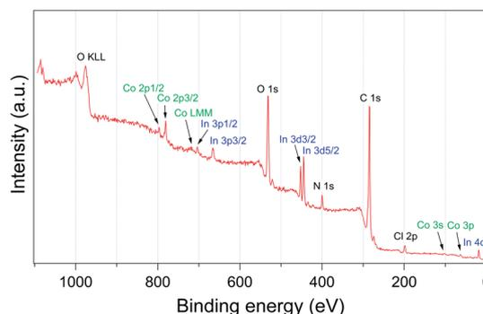
Fig. 3 Survey XPS spectrum of *trans*-[Co(en)<sub>2</sub>Cl<sub>2</sub>]<sup>+</sup>@InBTB.
