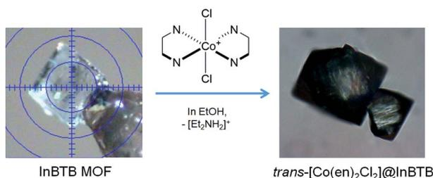
Fig. 1 Schematic of the preparation of  $\text{trans}[\text{Co}(\text{en})_2\text{Cl}_2]\text{Cl}$  into  $\text{trans}[\text{Co}(\text{en})_2\text{Cl}_2]\text{Cl}$  through the cation-exchange of  $[\text{Et}_4\text{NH}]^+$  with  $\text{trans}[\text{Co}(\text{en})_2\text{Cl}_2]^+$ .
