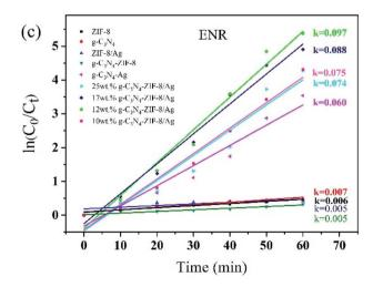
Fig. 7 (a) Degradation of antibiotics by the different materials under visible light irradiation, (b) photocatalytic degradation performance at different times and (c) kinetic linear fitting curves of enrofloxacin under different materials.
