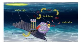
Fig. 11 Proposed photocatalysis mechanism of the  $Ag@ZIF-8/g-C_3N_4$  Z-scheme heterojunction.
