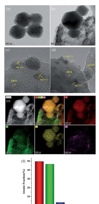
Fig. 3 TEM images of (a) Ag@ZIF-8 and (b-d) Ag@ZIF-8/g- $C_3N_4$ , (e) EDS spectrum of Ag@ZIF-8/g- $C_3N_4$  and (f) atomic percentages of Ag@ZIF-8/g- $C_3N_4$ .
