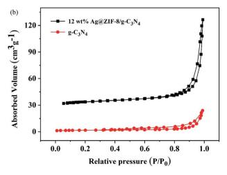
Fig. 4 Adsorption–desorption isotherms of (a) ZIF-8, Ag@ZIF-8, (b) g-  $C_3N_4$ , 12 wt% Ag@ZIF-8/g- $C_3N_4$ .
