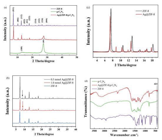
Fig. 1 XRD patterns of (a) ZIF-8,  $g-C_3N_4$  and Ag@ZIF-8/ $g-C_3N_4$ , (b) ZIF-8 and Ag@ZIF-8 with different Ag contents and (c) enlarged view of ZIF-8 and Ag@ZIF-8. (d) FT-IR spectra of Ag@ZIF-8,  $g-C_3N_4$  and Ag@ZIF-8/ $g-C_3N_4$ .
