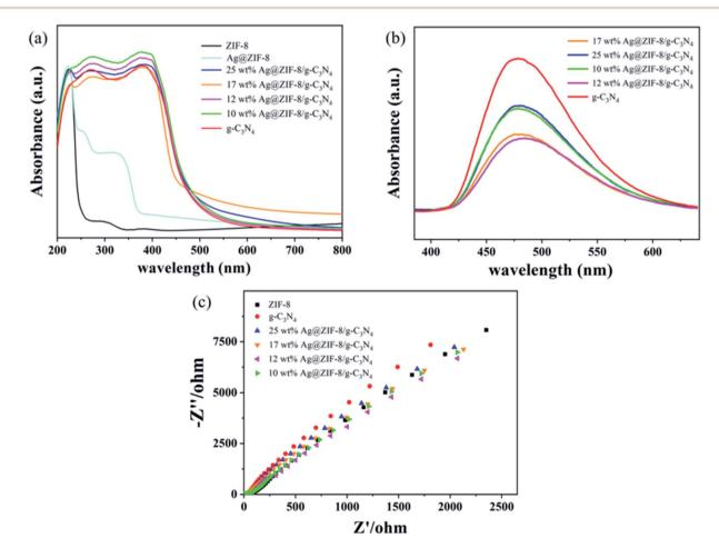
Fig. 6 (a) UV-vis diffuse reflectance spectra of pure  $g-C_3N_4$ , ZIF-8 and Ag@ZIF-8/ $g-C_3N_4$  with different  $g-C_3N_4$  contents, (b) PL spectra of pure  $g-C_3N_4$  and Ag@ZIF-8/ $g-C_3N_4$  with different  $g-C_3N_4$  with different  $g-C_3N_4$  with different  $g-C_3N_4$  contents and (c) EIS of ZIF-8, pure  $g-C_3N_4$  and Ag@ZIF-8/ $g-C_3N_4$  with different  $g-C_3N_4$  contents.
