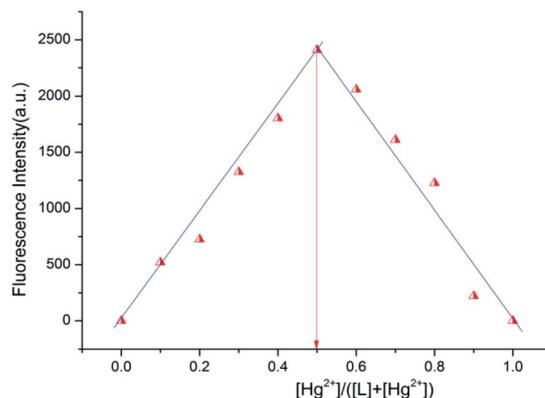
Fig. 5 Job's plot for determining the stoichiometry between L and Hg<sup>2+</sup> ion in CH<sub>3</sub>OH–H<sub>2</sub>O (4 : 1, v/v, Tris–HCl buffer pH = 8.0).
