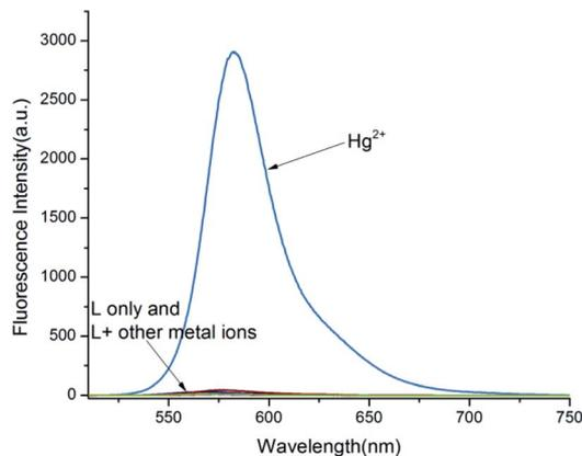
Fig. 2 Fluorescence responses of probe L upon treated with 10 equiv. metal ions in CH<sub>3</sub>OH–H<sub>2</sub>O (4 : 1, v/v, Tris–HCl buffer pH = 8.0).
