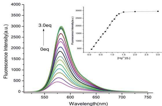
Fig. 4 Fluorescence emission spectra of probe L in the presence of various concentrations of Hg<sup>2+</sup> (0–3 equiv.) in CH<sub>3</sub>OH–H<sub>2</sub>O (4 : 1, v/v, Tris–HCl buffer pH = 8.0).
