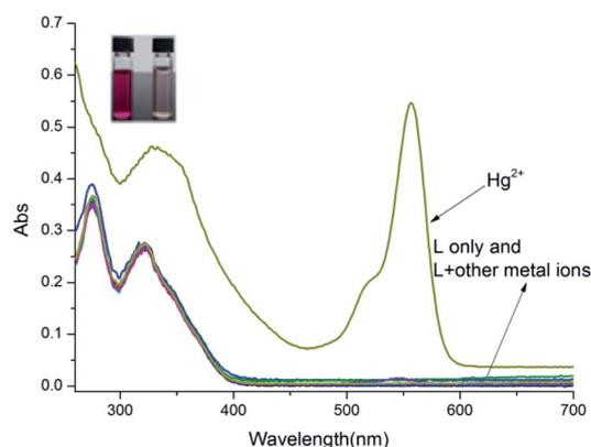
Fig. 1 The UV-vis absorption spectra changes of **L** (10  $\mu\text{M}$ ) in  $\text{CH}_3\text{OH}-\text{H}_2\text{O}$  (4 : 1, v/v, Tris-HCl buffer pH = 8.0) upon being treated with 10 equiv. metal ions.
