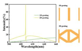
Fig. 3 Comparing the reflection spectra of one-dimensional gratings (1D) and two-dimensional (2D) gratings; the small images represent the structure of a single period on the x-y plane. Other parameters are consistent with those in Fig. 1.
