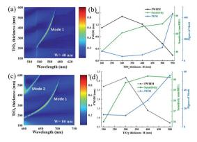
Fig. 5 Effect of  ${\rm TiO_2}$  nanostructure thickness on sensing performance. At a fixed grating width (a and b) W=40 nm and (c and d) W=40 nm,  ${\rm TiO_2}$  thickness is a function of wavelength, and FWHM, S, and FOM are functions of  ${\rm TiO_2}$  thickness. When the thickness of  ${\rm TiO_2}$  changes, the other parameters are consistent with those in Fig. 1.
