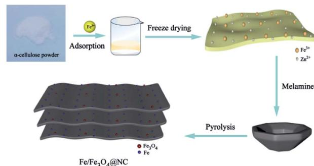
Scheme 1 Schematic diagram of Fe/Fe<sub>3</sub>O<sub>4</sub>@NC preparation process.
