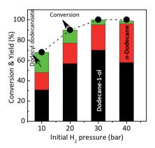
Fig. 4 Effect of initial  $H_2$  pressure on the conversion and yield in the hydroconversion of lauric acid over  $Ru-(0.026)MoO_x/TiO_2$  catalyst. Reaction conditions: catalyst, 0.065 g; lauric acid, 3.2 mmol; solvent, 2-propanol:  $H_2O$ , 5.0 ml (4.0 : 1.0 volume ratio); 170 °C, 7 h.
