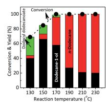
Fig. 3 Effect of reaction temperature on the conversion and yield in the hydroconversion of lauric acid over Ru–(0.026)MoO $_x$ /TiO $_2$  catalyst. Reaction conditions: catalyst, 0.065 g; lauric acid, 3.2 mmol; solvent, 2-propanol: H $_2$ O, 5.0 mL (4.0 : 1.0 volume ratio); H $_2$  40 bar, 7 h
