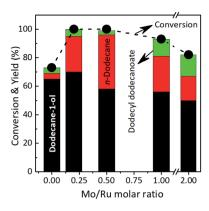
Fig. 1 Results of product distribution (yield) from selective hydroconversion of lauric acid using Ru–MoO $_x$ /TiO $_2$  catalysts with different Mo loading amounts. Reaction conditions: catalyst, 0.065 g; lauric acid, 3.2 mmol; solvent, 2-propanol: H $_2$ O, 5 mL (4.0:1.0 volume ratio); H $_2$  40 bar, 170 °C, 7 h.
