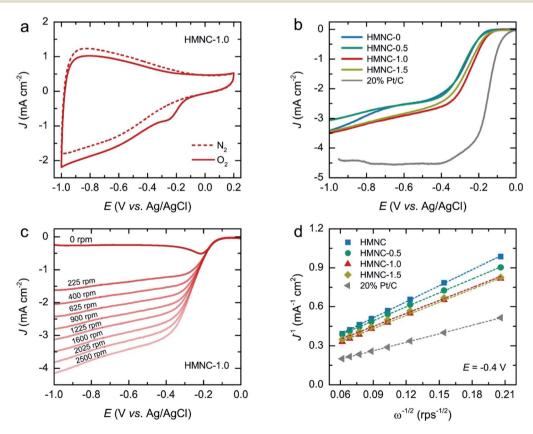
Fig. 6 Electrochemical measurements for ORR: (a) CV curve of HMNC-1.0 measured in  $N_2$  and  $O_2$ -saturated 0.1 M KOH solution (50 mV s<sup>-1</sup>), (b) LSV curves of all catalysts at a rotation speed of 1600 rpm (10 mV s<sup>-1</sup>), (c) LSV curves measured at different rotation speeds from 0 to 2500 rpm of HMNC-1.0, and (d) the K-L plots obtained from a series of LSV curves at different rotation speeds of all catalysts at a potential of -0.4 V.
