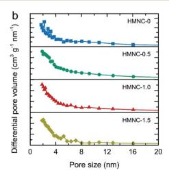
Fig. 3 Surface area and porosity analyses: (a) N<sub>2</sub> adsorption–desorption isotherms and (b) BJH pore size distribution of HMNCs.
