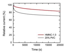
Fig. 7 Chronoamperometric response of HMNC-1.0 and 20% Pt/C measured at an applied potential of -0.4 V (1600 rpm) in O<sub>2</sub>-saturated 0.1 M KOH solution.
