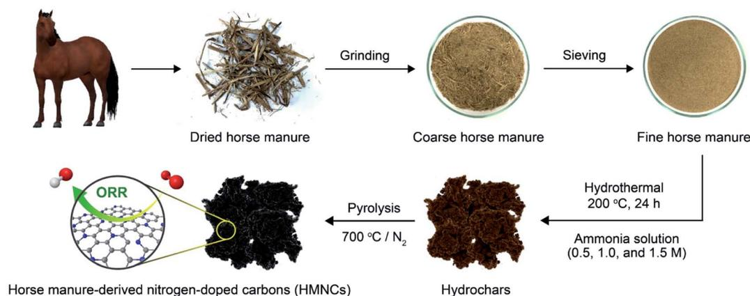
Fig. 1 Schematic illustration illustrating the synthesis of HMNCs in this work.
