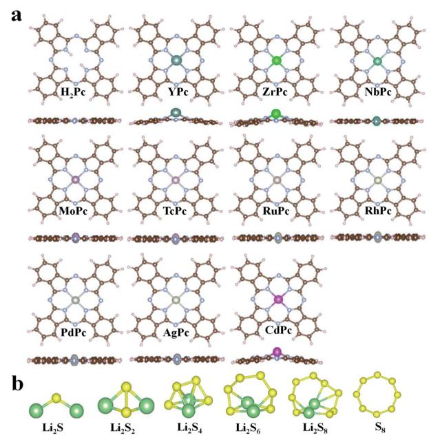
Fig. 1 (a) The schematic diagram of the optimized  $H_2Pc^{24}$  and TMPc structures. (b) The fully relaxed  $Li_2S_1$ ,  $Li_2S_2$ ,  $Li_2S_3$ ,  $Li_2S_4$ ,  $Li_2S_6$ ,  $Li_2S_8$  and  $Li_2S_8$
