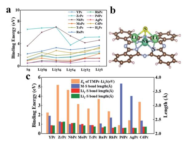
Fig. 2 (a) Binding energy of  $S_8/Li_2S_x$  (x=1, 2, 4, 6, 8) adsorbed on different  $H_2Pc^{24}/TMPc$  surfaces; (b) the schematic diagram of NbPc-Li<sub>2</sub>S binding system with atomic label (Li<sub>1</sub>, Li<sub>2</sub>, S, Nb and N atoms); (c) the binding energy, TM-S bond lengths and Li<sub>1/2</sub>-S bond lengths histogram of different TMPc-Li<sub>2</sub>S systems.
