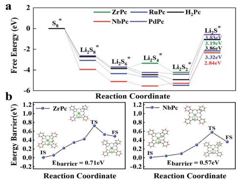
Fig. 5 (a) Relative free energy profiles for the discharging process from  $S_8$  to  $Li_2S$  on the ZrPc, NbPc, RuPc, PdPc and  $H_2$ Pc surfaces. (b) The decomposition free energy barriers of the  $Li_2S$  on ZrPc and NbPc surfaces, and the corresponding initial, transition, and final structures are shown in the illustration.
