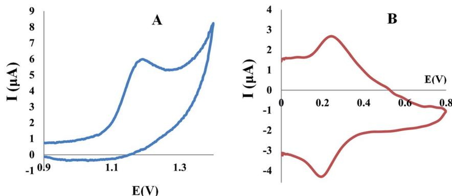
Fig. 6 (A) Cyclic voltammogram of  $1.00 \times 10^{-3}$  M TAM, (B) cyclic voltammogram of  $1.00 \times 10^{-3}$  M SOL at Al<sub>2</sub>O<sub>3</sub>-NPs/MWCNTs/CPE in BR buffer (0.04 M) pH 4.0 and scan rate of 100 mV s<sup>-1</sup>.
