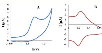
Fig. 6 (A) Cyclic voltammogram of  $1.00 \times 10^{-3}$  M TAM, (B) cyclic voltammogram of  $1.00 \times 10^{-3}$  M SOL at Al<sub>2</sub>O<sub>3</sub>-NPs/MWCNTs/CPE in BR buffer (0.04 M) pH 4.0 and scan rate of 100 mV s<sup>-1</sup>.
