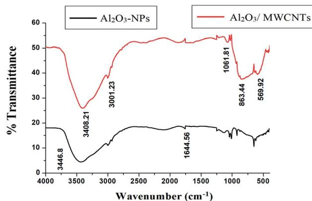
Fig. 2 FTIR spectra of MWCNTs and Al<sub>2</sub>O<sub>3</sub>-NPs/MWCNTs.
