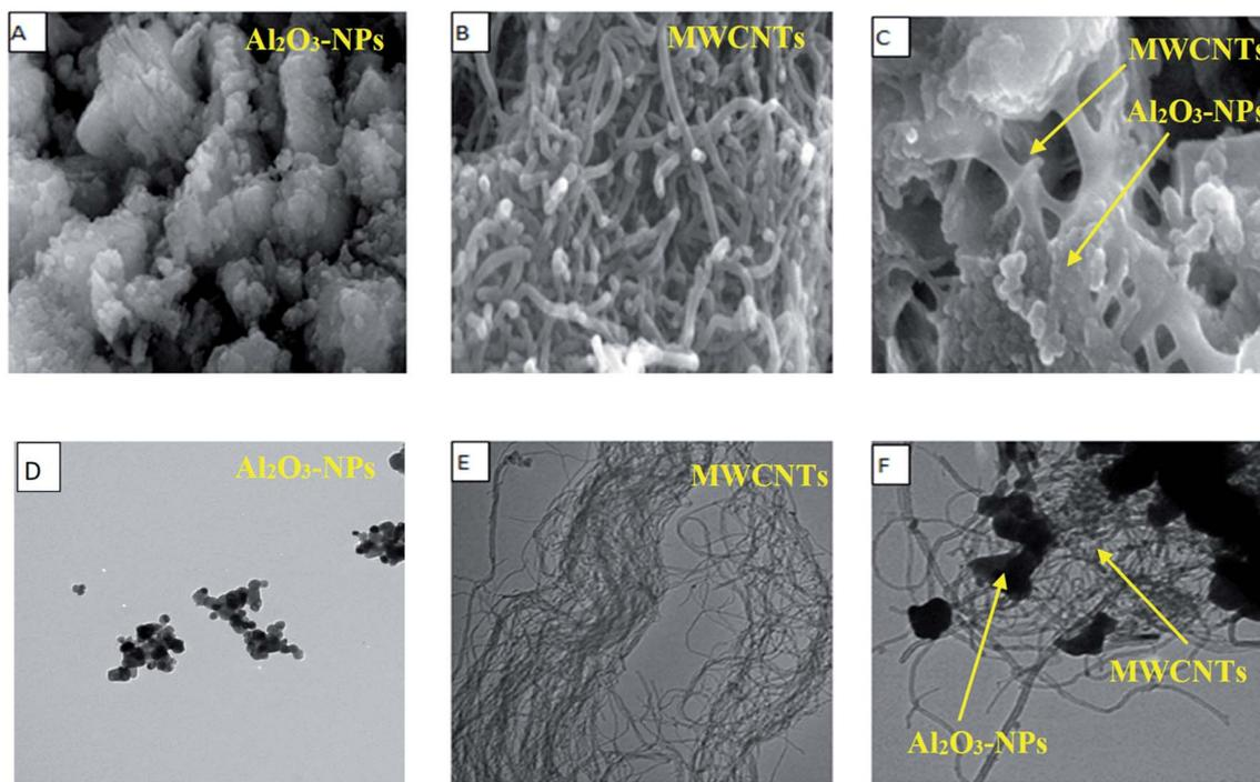
Fig. 1 (A) SEM image, (B) MWCNTs SEM image, (C) Al<sub>2</sub>O<sub>3</sub>-NPs/MWCNTs SEM image, (D) Al<sub>2</sub>O<sub>3</sub>-NPs TEM image, (E) MWCNTs TEM image, (F) Al<sub>2</sub>O<sub>3</sub>-NPs/MWCNTs TEM image.
