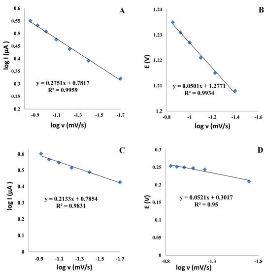
Fig. 8 The log scan rate ( $\nu$ ) versus the log peak current  $I_p$  and the potential E of TAM (A and B) and SOL (C and D) at Al $_2$ O $_3$ -NPs/MWCNTs/CPE.
