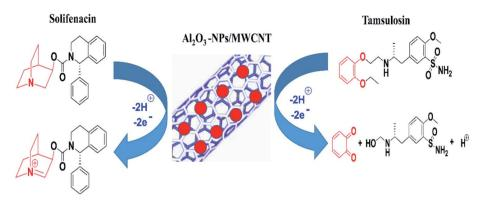
Scheme 1 Proposed oxidation mechanisms of tamsulosin & solifenacin and sensor configuration.
