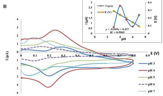
Fig. 7 The pH effect on the potential and peak current of TAM (A) and SOL (B) in BR buffer (0.04 M) pH 4.0.
