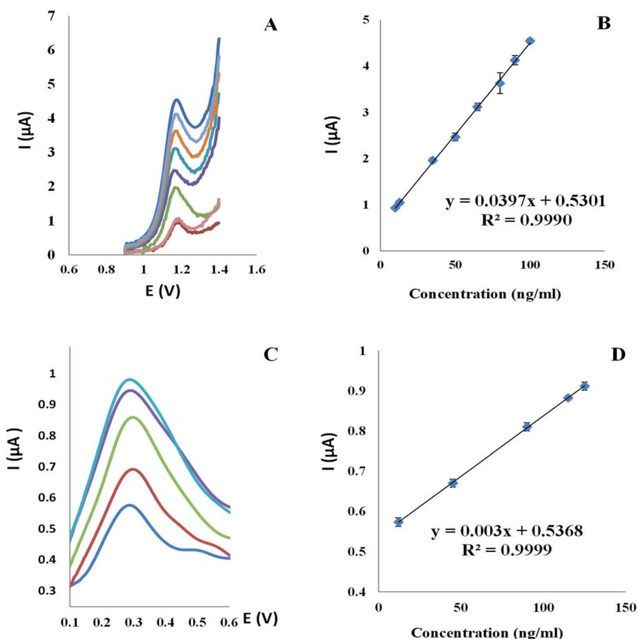
Fig. 9 (A) Square wave voltammograms and (B) the corresponding calibration curve for TAM concentrations range (10 to 100 ng ml<sup>-1</sup>) and (C) square wave voltammograms and (D) the corresponding calibration curve for SOL concentrations range (12 to 125 ng ml<sup>-1</sup>) at Al<sub>2</sub>O<sub>3</sub>-NPs/MWCNTs/CPE in BR buffer (0.04 M) pH 4.0 and scan rate of 100 mV s<sup>-1</sup>.
