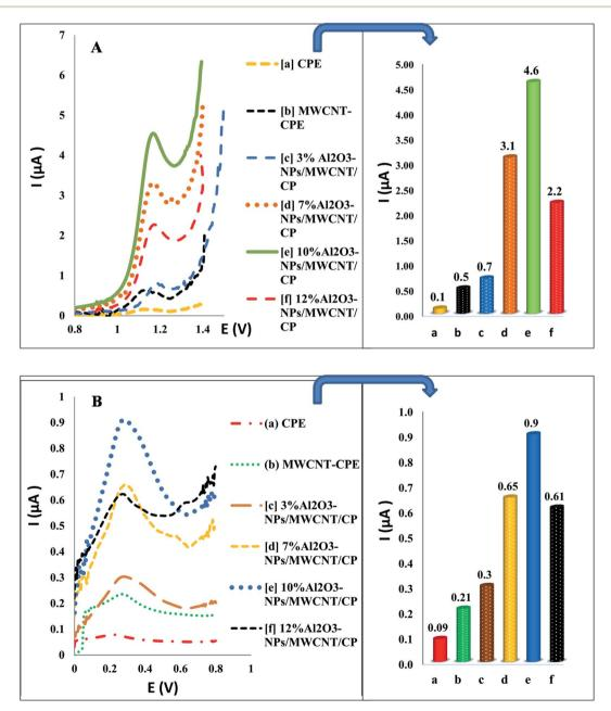
Fig. 5 The Al<sub>2</sub>O<sub>3</sub>-NPs contents and different electrodes effect on oxidation peak height of TAM (A) and SOL (B) using SWV.
