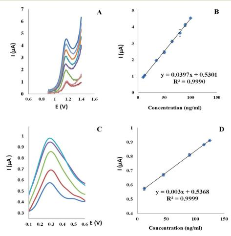
Fig. 9 (A) Square wave voltammograms and (B) the corresponding calibration curve for TAM concentrations range (10 to 100 ng ml $^{-1}$ ) and (C) square wave voltammograms and (D) the corresponding calibration curve for SOL concentrations range (12 to 125 ng ml $^{-1}$ ) at Al<sub>2</sub>O<sub>3</sub>-NPs/MWCNTs/CPE in BR buffer (0.04 M) pH 4.0 and scan rate of 100 mV s $^{-1}$ .
