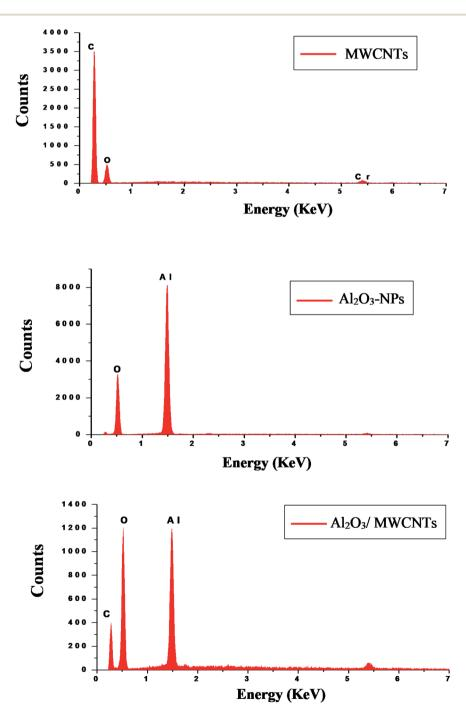
Fig. 3 EDX patterns of MWCNTs, Al<sub>2</sub>O<sub>3</sub>-NPs, and Al<sub>2</sub>O<sub>3</sub>-NPs/MWCNTs.
