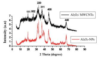
Fig. 4 XRD patterns of Al<sub>2</sub>O<sub>3</sub>-NPs and Al<sub>2</sub>O<sub>3</sub>-NPs/MWCNTs.
