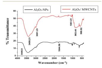
Fig. 2 FTIR spectra of MWCNTs and Al<sub>2</sub>O<sub>3</sub>-NPs/MWCNTs.
