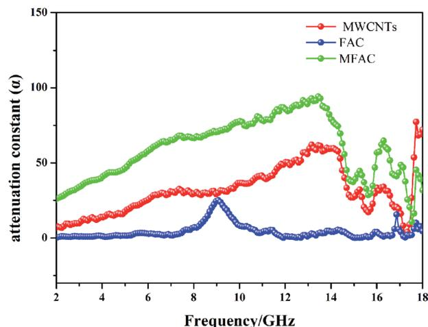
Fig. 9 Attenuation constant of all the samples.
