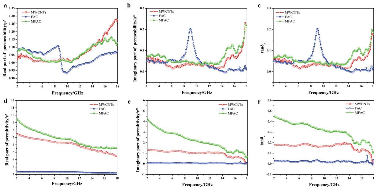
Fig. 5 (a) Real parts ( $\mu'$ ) and (b) imaginary parts ( $\mu''$ ) of complex permeability of MWCNTs, FACs and MFACs. (d) Real parts ( $\epsilon'$ ) and (e) imaginary parts ( $\epsilon''$ ) of complex permittivity of corresponding samples. (c) Magnetic loss tangent and (f) dielectric loss tangent of corresponding samples versus frequency.
