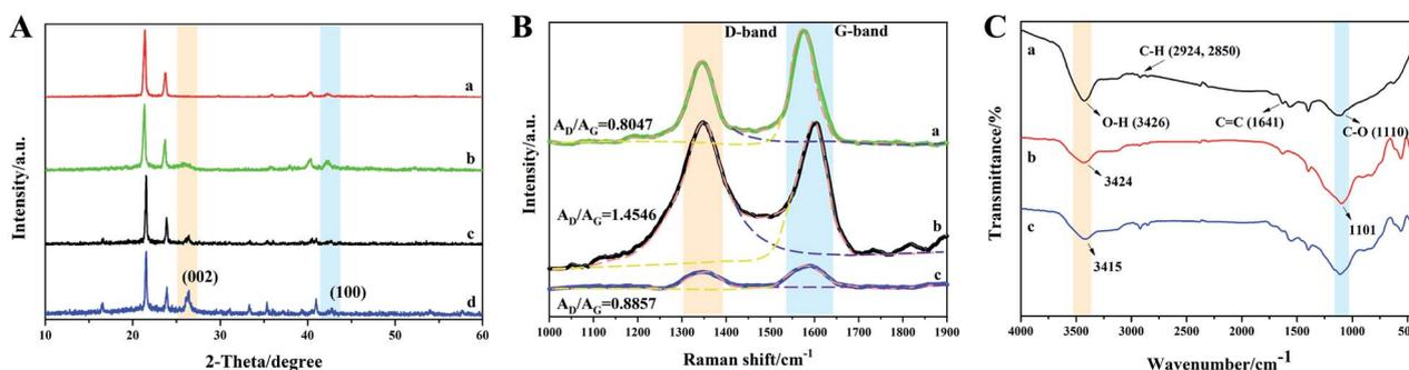
Fig. 3 (A) XRD patterns of the ring used to characterize the EMW absorption properties: (a) pure paraffin wax, (b) MWCNTs, (c) FACS, and (d) MFACs. (B) Raman spectra and (C) FT-IR spectra of samples without paraffin wax: (a) MWCNTs, (b) FACS, and (c) MFACs.
