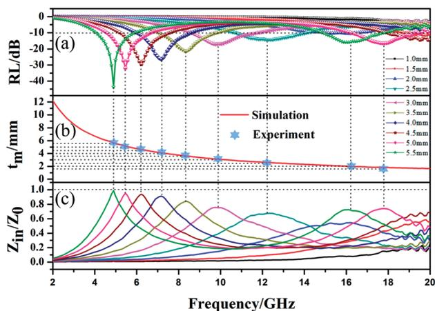
Fig. 8 (a) RL–F curves, (b) relationship between simulated thickness and peak frequency, and (c) relationship between  $Z_{in}/Z_0$  and EMW frequency of MFACs.
