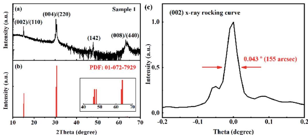
Fig. 2 Structural properties of as-grown CsPbBr<sub>3</sub> single crystal. Powder XRD patterns of (a) as-grown CsPbBr<sub>3</sub> single crystal and (b) CsPbBr<sub>3</sub> bulk material obtained from PDF card: 01-072-7929. (c) (002) XRC curve of as-grown CsPbBr<sub>3</sub> single crystal.
