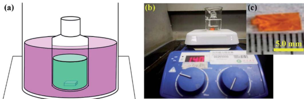
Fig. 1 Growth of  $\text{CsPbBr}_3$  single crystal. (a) Schematic illustration of experimental setup. Optical images of  $\text{CsPbBr}_3$  single crystal captured (b) during the growth and (c) at the end of growth.
