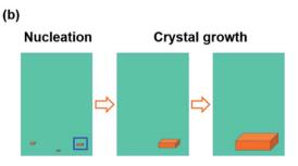
Fig. 5 (a) Calculated steady-state temperature field distribution of the precursor solution (labeled as solution 1) heated on the hot table with an oil bath (labeled as solution 2). (b) Proposed growth process of CsPbBr<sub>3</sub> single crystal.
