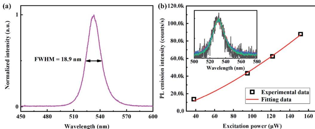
Fig. 3 Optical properties of as-grown CsPbBr<sub>3</sub> single crystal. (a) RT PL spectrum of as-grown CsPbBr<sub>3</sub> single crystal. (b) Excitation power dependence of PL emission intensities of as-grown CsPbBr<sub>3</sub> single crystal. The inset in (b) shows the normalized PL spectrum captured under different excitation power.
