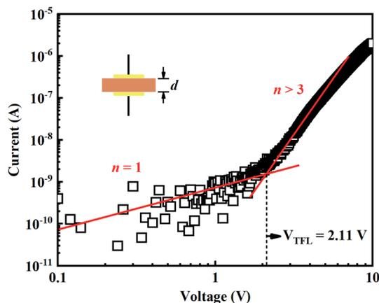
Fig. 4  $I$ - $V$  curve of an Au/CsPbBr<sub>3</sub>/Au structured device. The  $I$ - $V$  curve is fitted using a power law ( $I \sim V^n$ ) (shown as red line).
