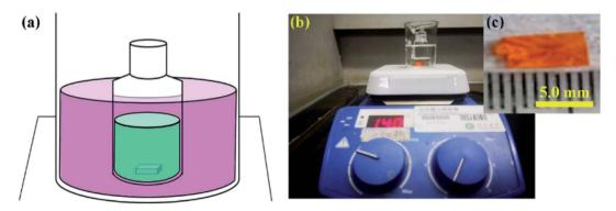
Fig. 1 Growth of CsPbBr<sub>3</sub> single crystal. (a) Schematic illustration of experimental setup. Optical images of CsPbBr<sub>3</sub> single crystal captured (b) during the growth and (c) at the end of growth.
