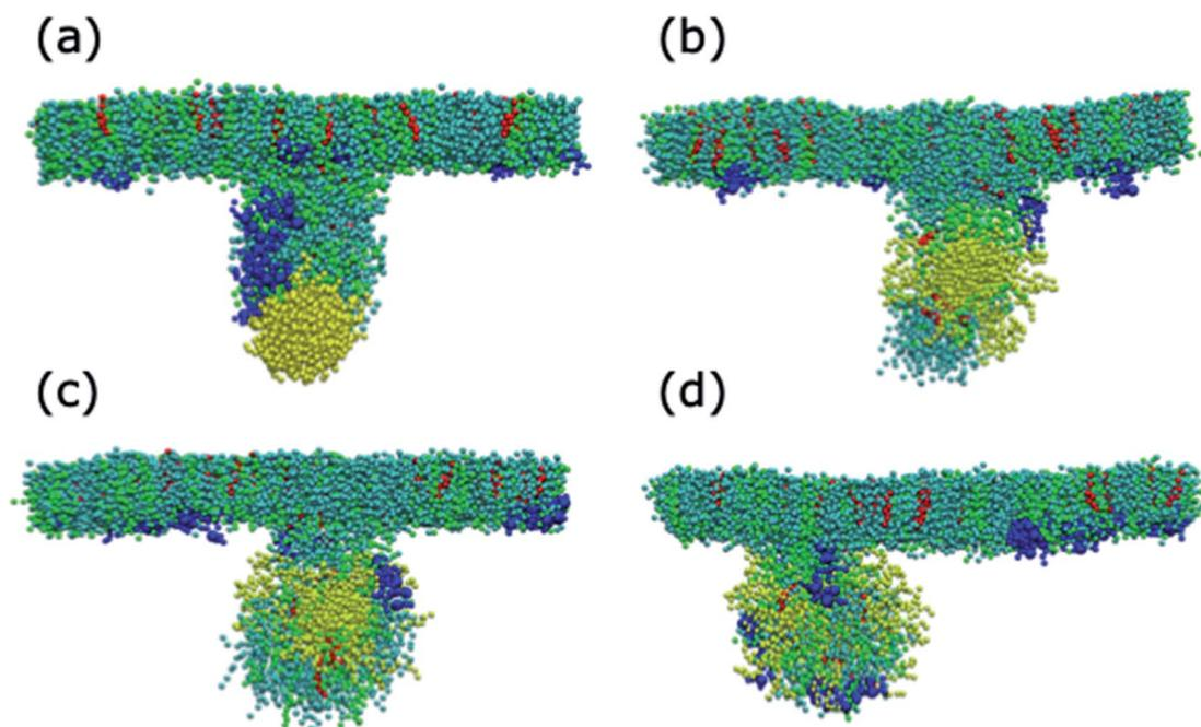
Fig. 6 Representative snapshots of the equilibrated systems with PS monolayers in the compressed system, the PEG-AuNPs have a chain density of 1.56 chain per nm<sup>2</sup> and a chain length of (a) 1, (b) 2, (c) 3 and (d) 4. DPPC, POPG, cholesterol, SP-B<sub>1-25</sub> and the PEG-AuNP are coloured cyan, green, red, blue and yellow, respectively.
