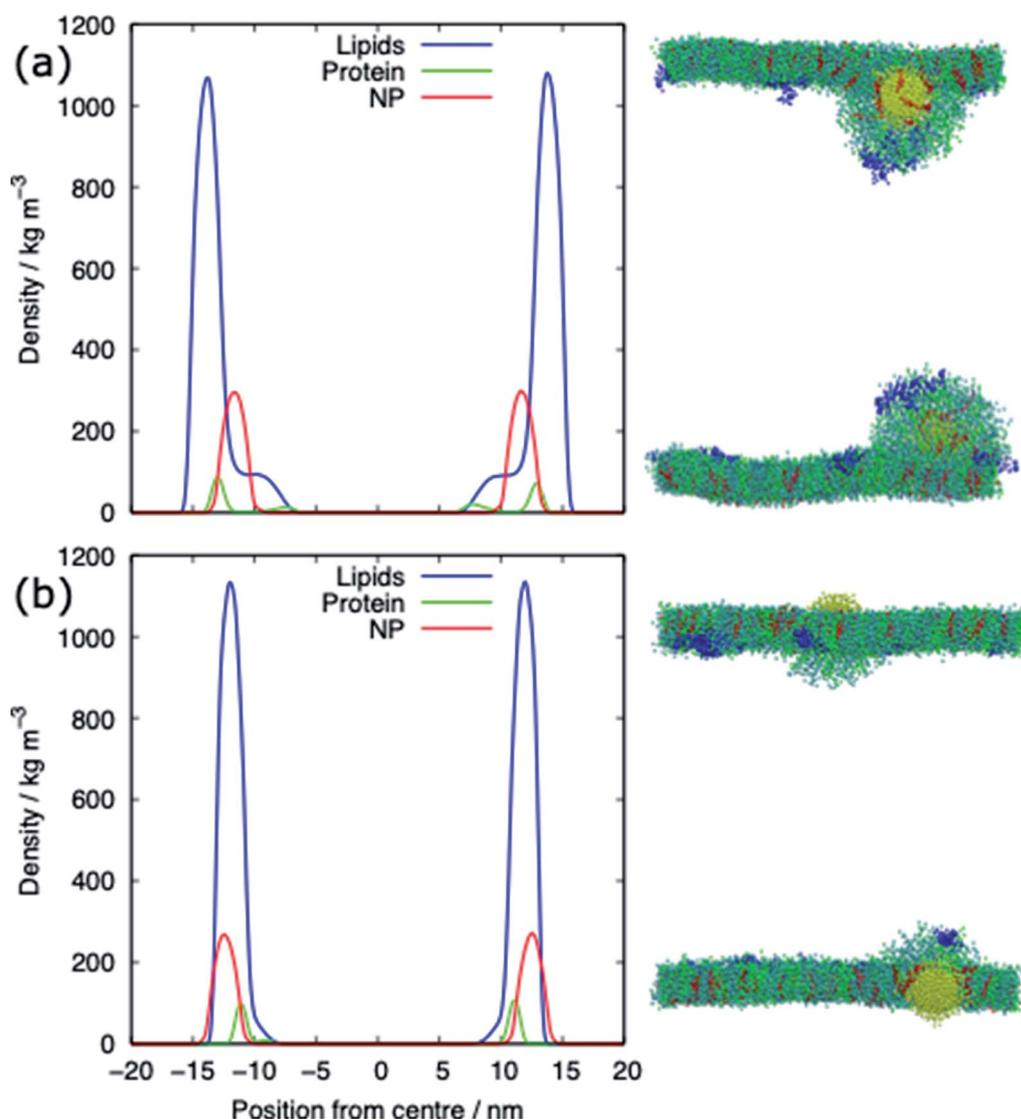
Fig. 4 Density profiles and representative snapshots of the alkyl-functionalised AuNP interacting with (a) the compressed (APL = 0.48 nm<sup>2</sup>) and (b) the expanded (APL = 0.54 nm<sup>2</sup>) phases. Data shown for the alkanethiol–AuNP with a chain density of 2.33 chain per nm<sup>2</sup> and a chain length of 2.
