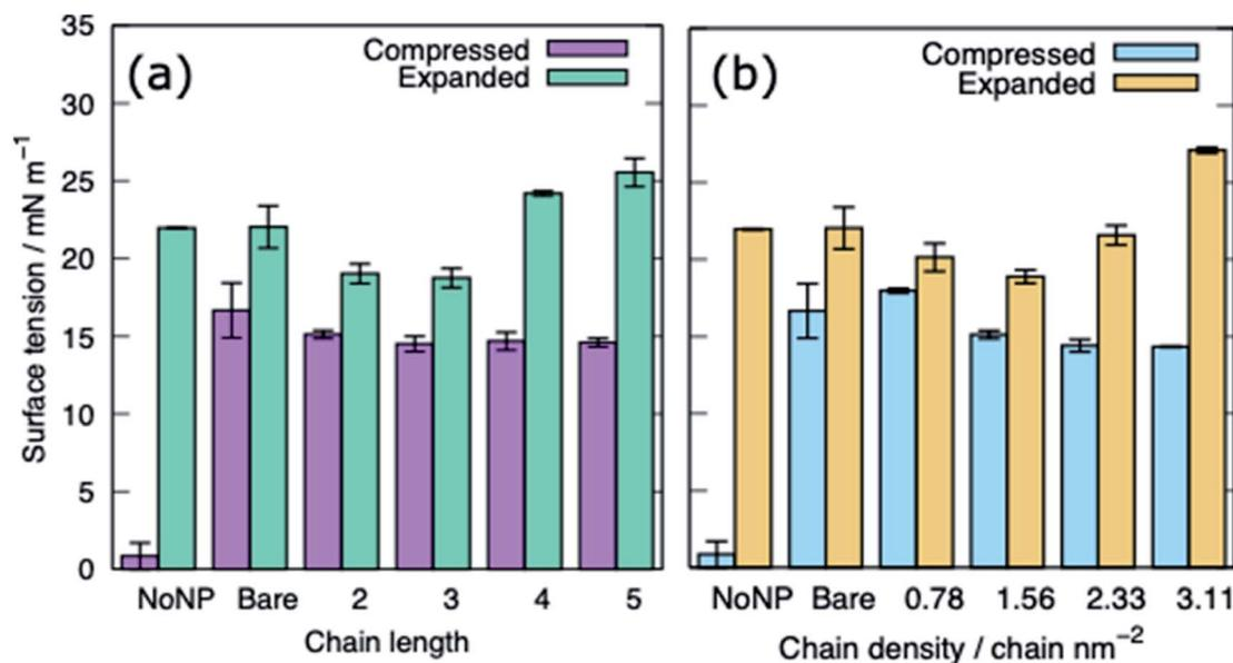
Fig. 5 The surface tension of PS monolayers in the presence of alkanethiol-functionalised AuNPs, data given for systems with APLs 0.48 and 0.54 nm<sup>2</sup>, (a) effect of varying ligand chain length (density = 2.33 chains per nm<sup>2</sup>), (b) effect of varying ligand chain density (length = 2). Bare refers to a system with bare AuNP.
