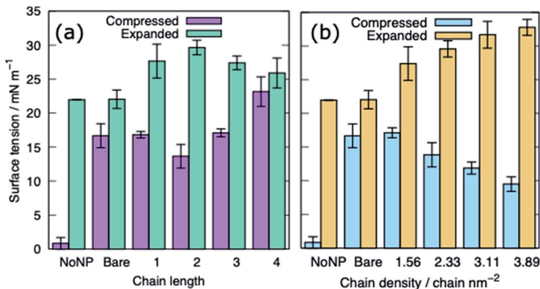
Fig. 8 The surface tension of PS monolayers in the presence of PEG-SH functionalised AuNPs for the compressed and expanded systems: (a) varying ligand chain length (density = 1.56 chains per  $\text{nm}^2$ ), (b) varying ligand chain density (length = 2). Bare refers to a system with a bare AuNP.
