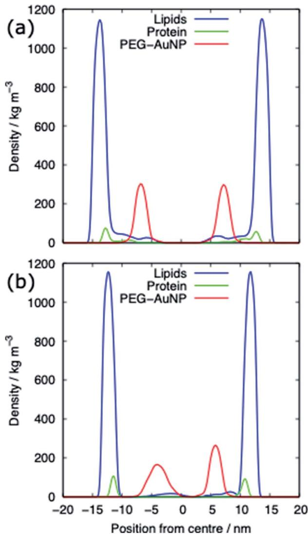
Fig. 7 Density profiles of the PEG-SH functionalised AuNP PS monolayer systems for (a) the compressed (APL = 0.48 nm $^2$ ) and (b) the expanded (APL = 0.54 nm $^2$ ) phase. Data shown for the PEG-AuNP with a chain density of 2.33 chain per nm $^2$  and a chain length of 2.
