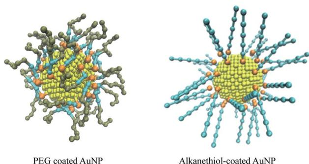
**Fig. 1** Structure of coarse-grained PEG-SH functionalised and alkanethiol-functionalised AuNP. The gold, sulfur, alkyl chain and ethyleneoxide sites are coloured yellow, orange, cyan and tan, respectively. The snapshots are of systems with a coating density of 1.56 chain per  $\text{nm}^2$ , with a chain length of 2 and 5 for the PEG and alkanethiol systems respectively.
