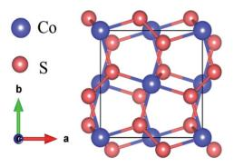
Fig. 1 The optimized structure of the bulk CoS<sub>2</sub>.
