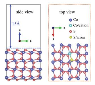
The crystallographic structure of CoS<sub>2</sub>(001) surface
