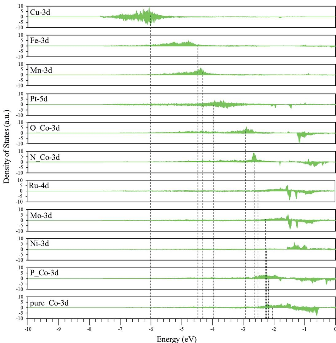
Fig. 5 The density of states at active metal sites. The dashed line marked the d-band center. The Fermi energy is set to zero.
