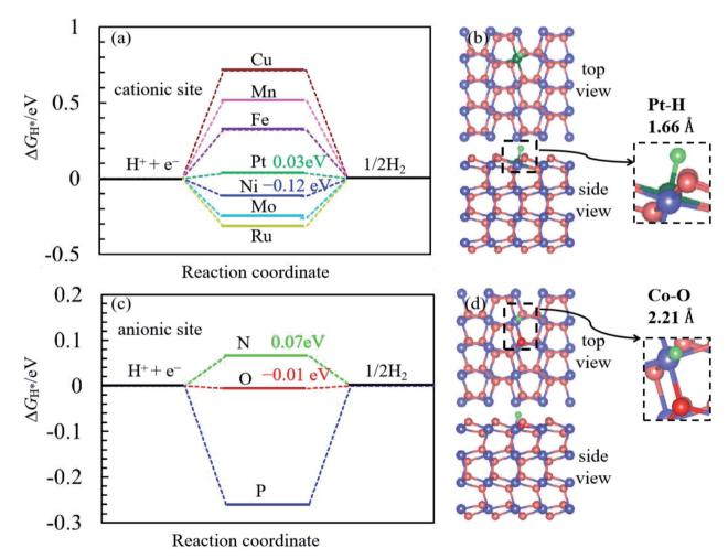
Fig. 4 (a) and (b) are  $\Delta G_{H^*}$  diagram and the structure of Pt-doped CoS<sub>2</sub>(001) with H adsorption at Pt site, respectively. (c) and (d) are  $\Delta G_{H^*}$  diagram and the structure of O-doped CoS<sub>2</sub>(001) with H adsorption at Co site, respectively. The blue, dark green, red balls and light green ball are Co, S, Pt, O and H atoms, respectively. Pt-H bond length is 1.66 Å and Co-O bond length is 2.21 Å.
