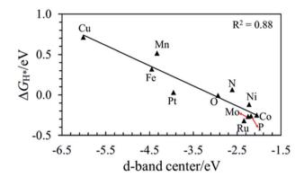
Fig. 6 The linear relationship between  $\Delta G_{H^*}$  and d-band centers of H adsorption sites.
