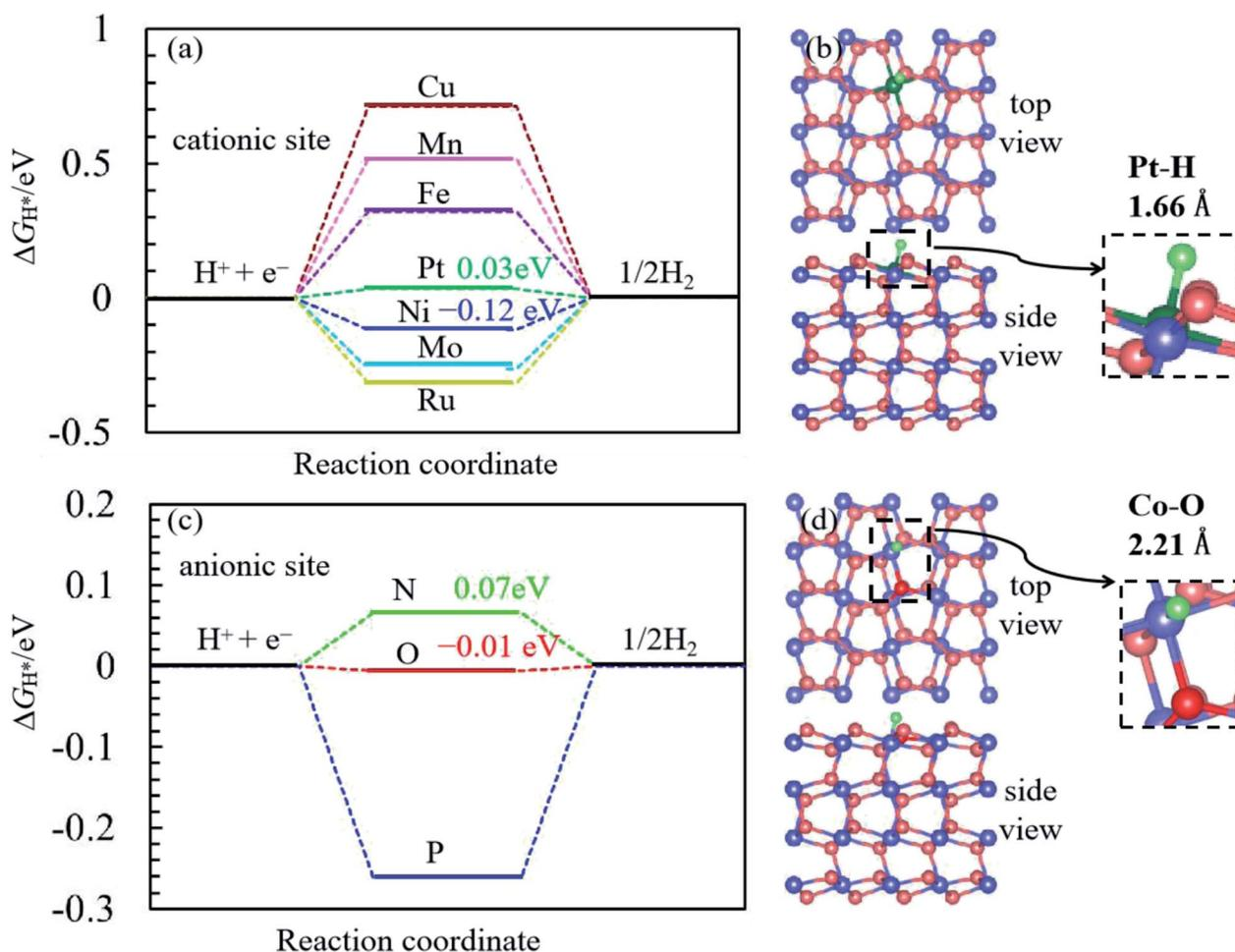
Fig. 4 (a) and (b) are  $\Delta G_{\text{H}^*}$  diagram and the structure of Pt-doped  $\text{CoS}_2(001)$  with H adsorption at Pt site, respectively. (c) and (d) are  $\Delta G_{\text{H}^*}$  diagram and the structure of O-doped  $\text{CoS}_2(001)$  with H adsorption at Co site, respectively. The blue, dark red, dark green, red balls and light green ball are Co, S, Pt, O and H atoms, respectively. Pt–H bond length is 1.66 Å and Co–O bond length is 2.21 Å.
