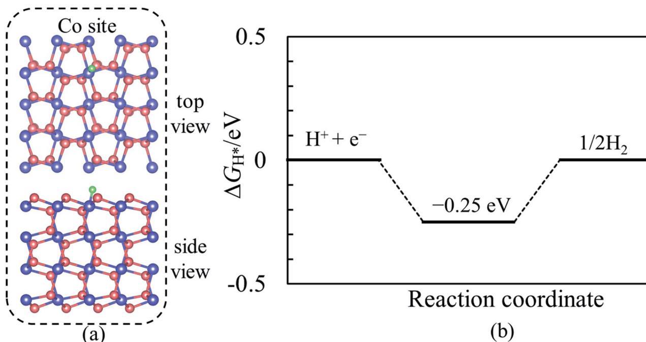
Fig. 3 (a) Represents the H adsorption structure of the pristine CoS<sub>2</sub>, where H adsorbs at Co site. The green ball refers to H atom. (b) is  $\Delta G_{H^*}$  diagram of the pristine CoS<sub>2</sub>.
