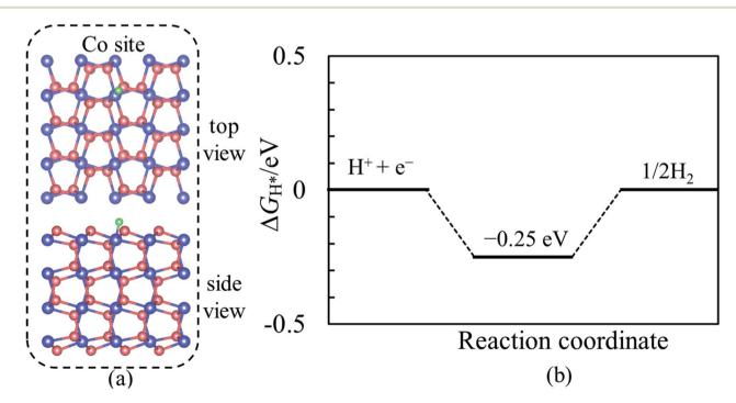
Fig. 3 (a) Represents the H adsorption structure of the pristine  $CoS_2$ , where H adsorbs at Co site. The green ball refers to H atom. (b) is  $\Delta G_{H^*}$  diagram of the pristine  $CoS_2$ .
