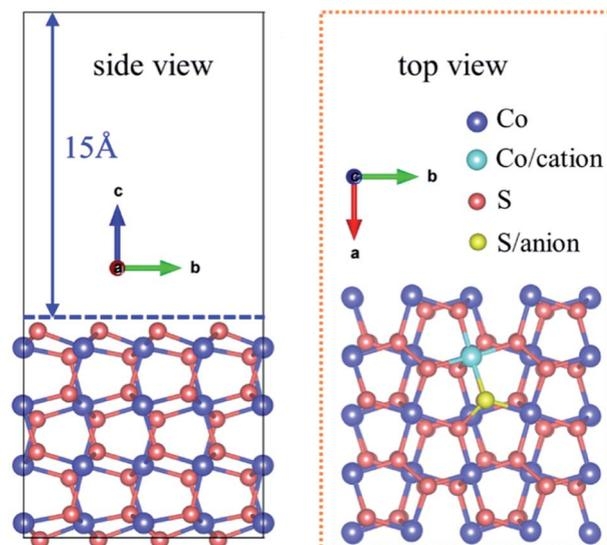
Fig. 2 The crystallographic structure of CoS<sub>2</sub>(001) surface.
