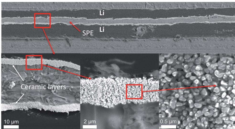
Fig. 7 SEM cross-section views of a LiAl/SPE/LiAl stack with a  $\sim 4 \mu\text{m}$  thick 85%  $\text{Al}_2\text{O}_3$ -sph ceramic layer on the surface of the lithium foil. The compact ceramic layers are well visible between the lithium foils and the SPE.
