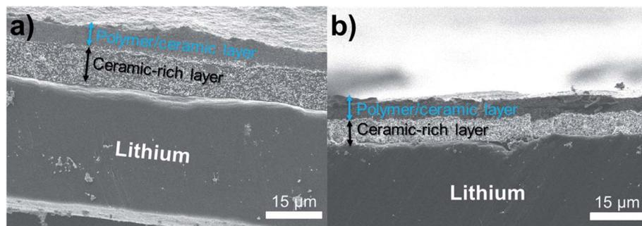
Fig. 4 SEM images of thick overcoatings deposited on LiAl surface and composed of: (a) 70%  $\text{Al}_2\text{O}_3$ -sph ( $\sim 15$ – $20 \mu\text{m}$ ) and (b) 85%  $\text{Al}_2\text{O}_3$ -sph ( $\sim 15 \mu\text{m}$ ). Two layers are well distinguishable: a polymer/ceramic (dark) and a ceramic-rich layers (bright). The contrast is more visible on SEM image (b) due to the high concentration of ceramic.
