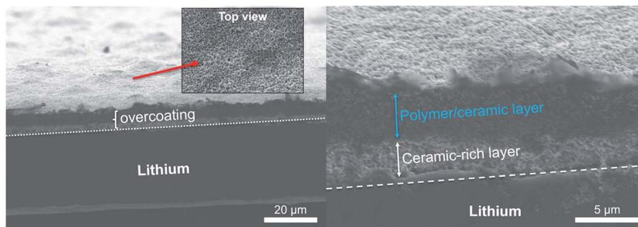
Fig. 2 SEM images showing an overcoating of 85%  $\text{Al}_2\text{O}_3$ -sph ( $\sim 6\text{--}7\ \mu\text{m}$ ) on the surface of LiAl. Two layers are well distinguishable: a polymer/ceramic and a ceramic-rich layers.
