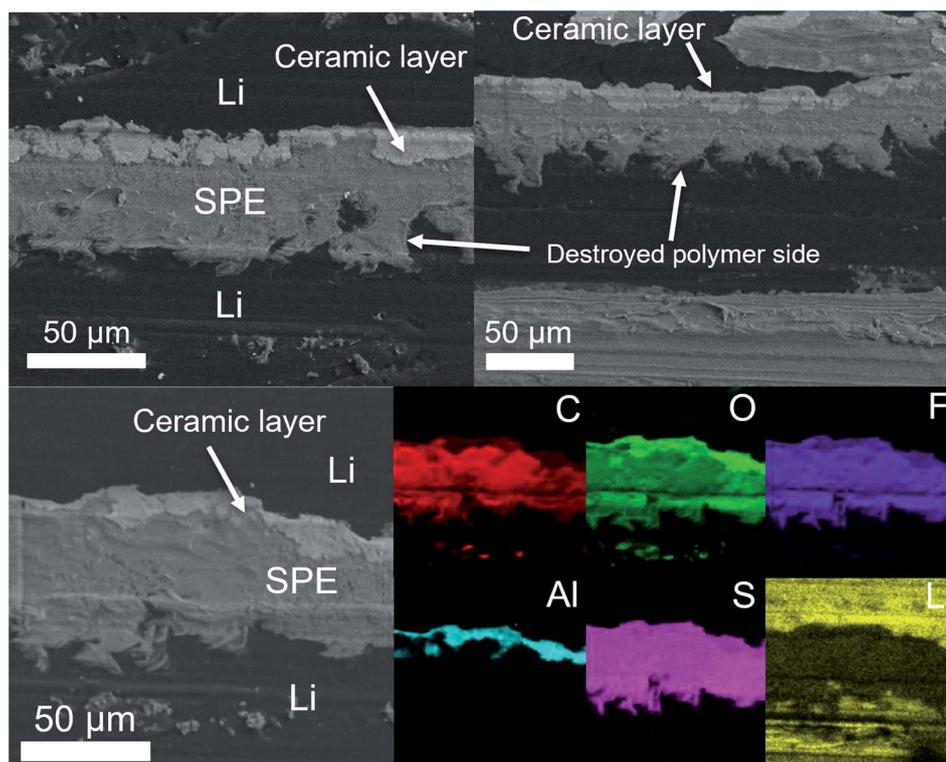
**Fig. 11** Cross-section view and corresponding elemental mapping of an asymmetric LiAl/SPE/LiAl stack with a  $\sim 5 \mu\text{m}$  thick 50%  $\text{Al}_2\text{O}_3$ -ndI ceramic layer on the surface of only one lithium foil. The cell assembled with this stack has been cycled at 1C for about 50 hours and during several hundreds of hours at different C-rates and then stopped before a short circuit happened.
