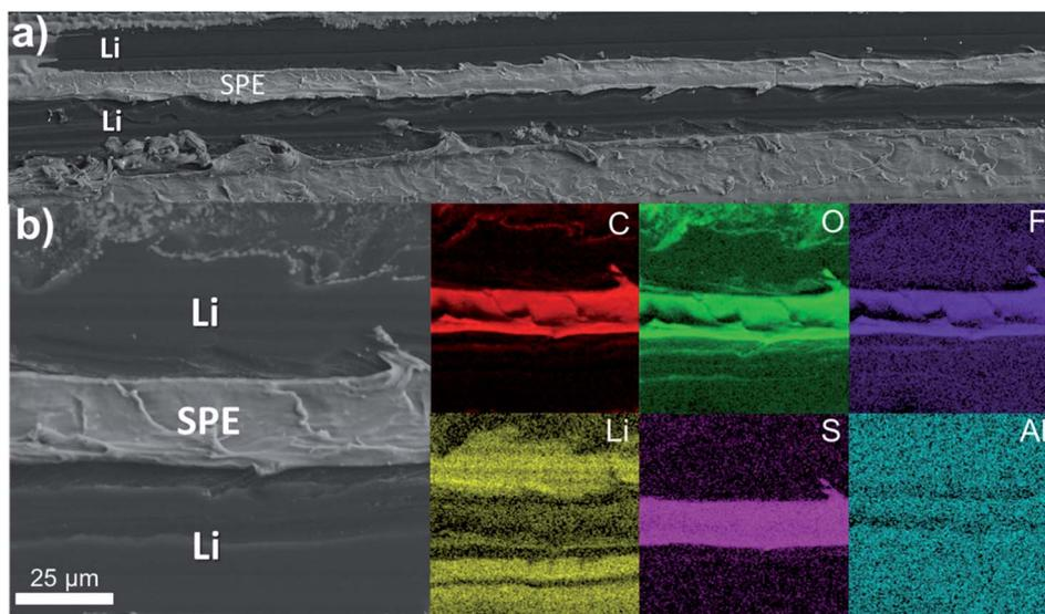
Fig. 5 (a and b) SEM cross-section views of a LiAl/SPE/LiAl stack with (b) the corresponding elemental mapping in C (red), O (green), F (purple), Li (yellow), S (pink) and Al (blue).
