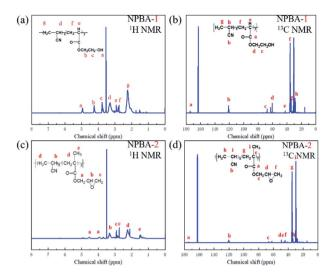
Fig. 1 (a) The <sup>1</sup>H NMR spectrum of NPBA-1 (b) <sup>13</sup>C NMR spectrum of NPBA-1 (c) the <sup>1</sup>H NMR spectrum of NPBA-2 (d) <sup>13</sup>C NMR spectrum of NPBA-2
