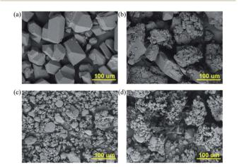
Fig. 3 The morphologies of HMX (a) before and (b) after coating with NPBA-2. The morphologies of RDX (c) before and (d) after coating with NPBA-2.
