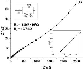
Fig. 11 EIS (electrochemical impedance spectroscopy): Nyquist plots of (a) mSi–P and (b) mSi  $\nu$ s. OC (open circuit) at 10 mV rms AC perturbation (in 1 M H<sub>2</sub>SO<sub>4</sub> electrolyte) with equivalent circuit diagram.
