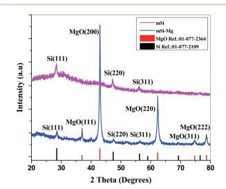
Fig. 3 X-ray diffractograms of mesoporous silicon reduced from mesoporous silica before (mSi-Mg) and after (mSi) the acid treatment.
