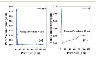
**Fig. 6** BJH pore size & volume analysis – Brunauer–Emmett–Teller (BET) of (a) SBA and (b) mSi by Halsey: Faas correction.
