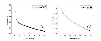
Fig. 13 GCCD (galvanostatic cyclic charge–discharge): discharge curve; potential vs. real time (a) mSi–P (at charge density =  $0.187 \text{ A g}^{-1}$ ) and (b) mSi (at charge density =  $0.210 \text{ A g}^{-1}$ ) in 1 M H<sub>2</sub>SO<sub>4</sub> electrolyte.
