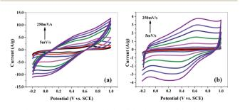
Fig. 8 Cyclic voltammogram (CV) of (a) mSi–P and (b) mSi at different scan rates on GCE in 1 M  $\rm H_2SO_4$  electrolyte vs. SCE.
