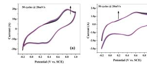
Fig. 9 Cyclic voltammetry (CV): cyclic stability of (a) mSi–P and (b) mSi at scan rate of 20 mV s $^{-1}$  for 50 cycles on GCE in 1 M H $_2$ SO $_4$  electrolyte vs. SCE.
