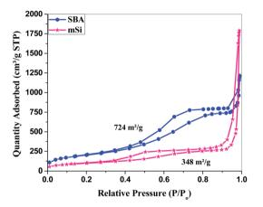
Fig. 5 Surface area analysis – Brunauer–Emmett–Teller (BET):  $N_2$  adsorption–desorption isotherm of SBA and mSi.
