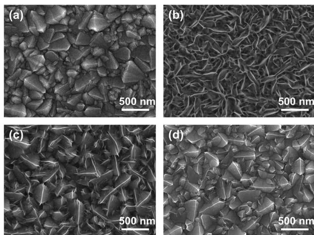
Fig. 2 Top-view SEM images of (a) NiO<sub>x</sub> film, and (b) 0-NiCo<sub>2</sub>O<sub>4</sub>, (c) 5-NiCo<sub>2</sub>O<sub>4</sub>, and (d) 10-NiCo<sub>2</sub>O<sub>4</sub> films deposited on FTO substrates.
