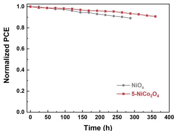
**Fig. 5** Long-term stability of the devices based on NiO<sub>x</sub> and 5-NiCo<sub>2</sub>O<sub>4</sub> HTLs stored at ambient conditions with humidity of 30–40%.
