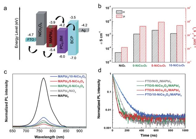
Fig. 3 (a) Energy band diagram relative to a vacuum level of the device. (BCP: bathocuproine) (b) Hall-effect measurements of NiO<sub>x</sub> and NiCo<sub>2</sub>O<sub>4</sub> films. (c) Steady-state photoluminescence of MAPbI<sub>3</sub> based on NiO<sub>x</sub> and NiCo<sub>2</sub>O<sub>4</sub> films. (d) Time-resolved photoluminescence spectra of the perovskite films on NiO<sub>x</sub> and NiCo<sub>2</sub>O<sub>4</sub> HTLs.
