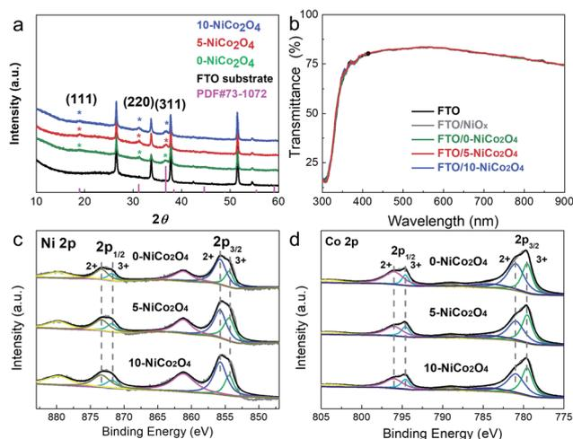
**Fig. 1** (a) XRD patterns of  $\text{NiCo}_2\text{O}_4$  films deposited on FTO/glass substrates, (b) optical transmission spectra of  $\text{NiO}_x$  and different  $\text{NiCo}_2\text{O}_4$  films, and XPS spectra of (c) Ni 2p and (d) Co 2p for the  $\text{NiCo}_2\text{O}_4$  films.
