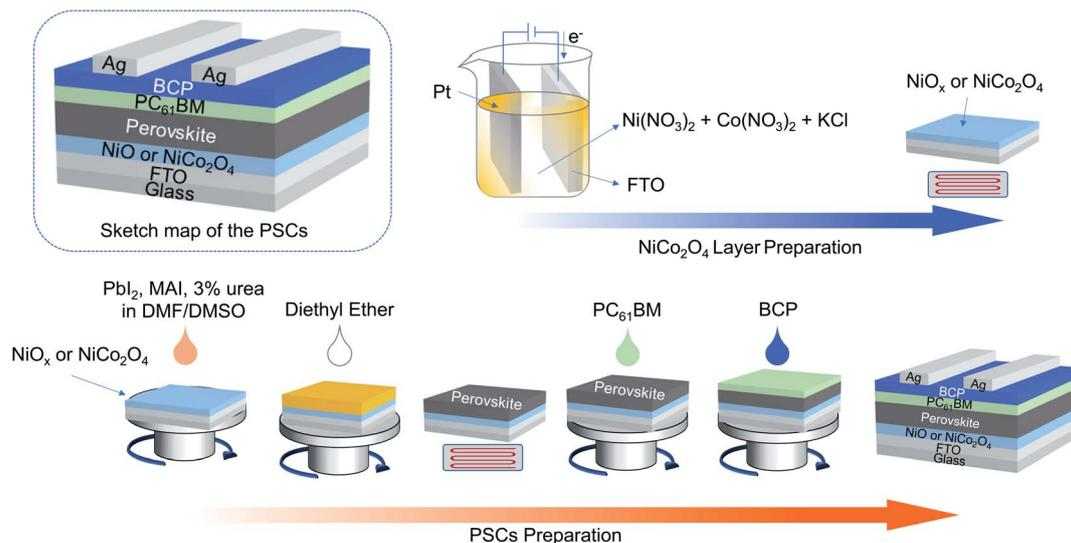
**Scheme 1** Schematic illustrations of  $\text{NiCo}_2\text{O}_4$  film fabrication process, prepared *via* electrochemical deposition, and of perovskite solar cell (PSC) preparation procedure. FTO: fluorine-doped tin oxide, DMF: dimethylformamide, DMSO: dimethyl sulfoxide.
