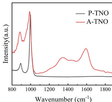
Fig. 5 Raman spectrum of A-TNO and P-TNO.
