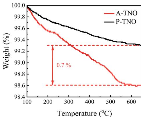
Fig. 6 TG analysis of A-TNO and P-TNO.
