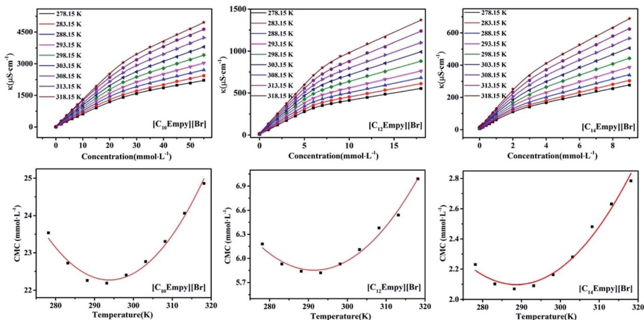
Fig. 4 The plot of conductivity vs. concentration of  $[C_n\text{Empy}][\text{Br}]$  at different temperatures and the curves of CMC value vs. temperature of  $[C_n\text{Empy}][\text{Br}]$  at different temperatures.
