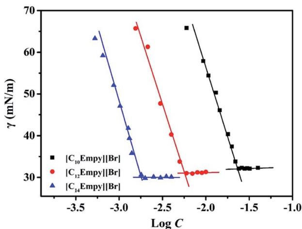
Fig. 3 The plot of surface tension against concentration of  $[C_n\text{Empy}][\text{Br}]$ .
