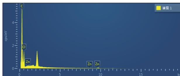
Fig. 8 EDX analysis of ZnO nanocomposite hydrogel.
