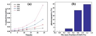
Fig. 12 (a) Electrical conductivity and (b) photosensitivity of ZnO nanocomposite hydrogels.
