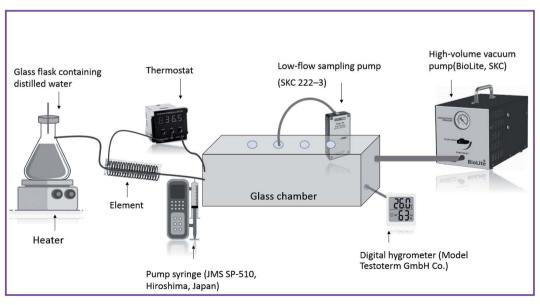
Fig. 1 Schematic diagram of the sampling chamber.
