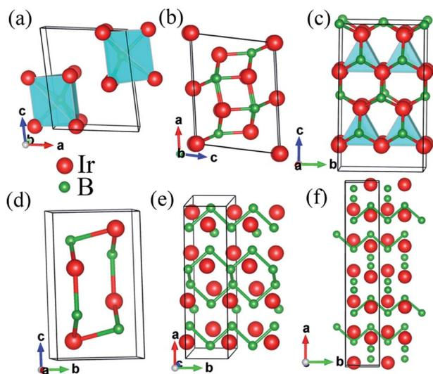
Fig. 2 Crystal structures of the six considered polymorphs at ambient pressure. (a)  $P2_1/m$ - $\text{Ir}_2\text{B}$ , (b)  $C2/m$ - $\text{Ir}_3\text{B}_2$ , (c)  $Fmm2$ - $\text{Ir}_4\text{B}_3$  (d)  $P2_1/m$ - $\text{IrB}$ , (e)  $Cm$ - $\text{Ir}_4\text{B}_5$  and (f)  $Pnma$ - $\text{Ir}_3\text{B}_4$ . The red and green spheres represent the Ir and B atoms, respectively.
