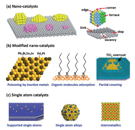
Fig. 6 Shapes of various nanocatalysts; (a) supported nanocatalyst, (b) modified nanocatalyst, and (c) single-atom catalyst (this figure has been adapted/reproduced from ref. 37 with permission from American Chemical Society, copyright 2019).
