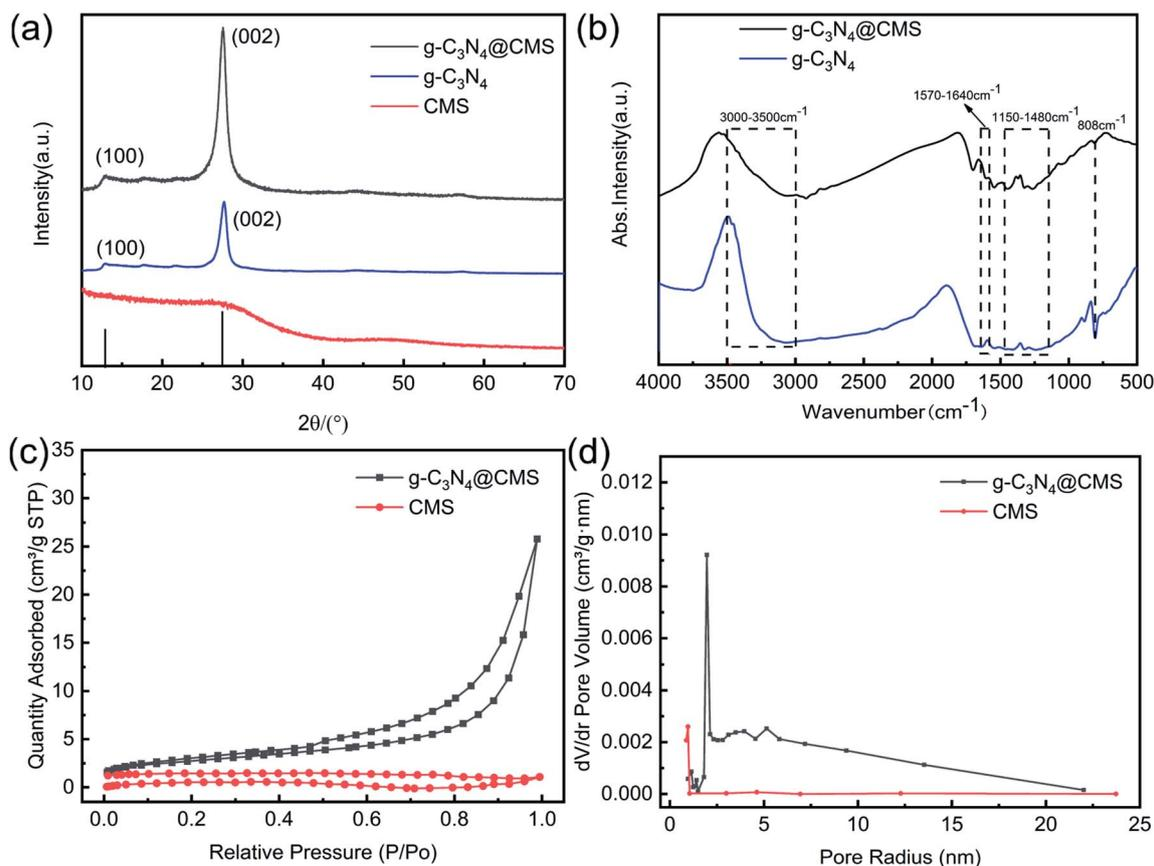
Fig. 3 (a) XRD patterns of g-C<sub>3</sub>N<sub>4</sub> and g-C<sub>3</sub>N<sub>4</sub>@CMS; (b) Fourier transform infrared spectra of g-C<sub>3</sub>N<sub>4</sub> and g-C<sub>3</sub>N<sub>4</sub>@CMS; (c) N<sub>2</sub> adsorption-desorption isotherms for CMS and g-C<sub>3</sub>N<sub>4</sub>@CMS; (d) pore size distribution of the CMS and g-C<sub>3</sub>N<sub>4</sub>@CMS.
