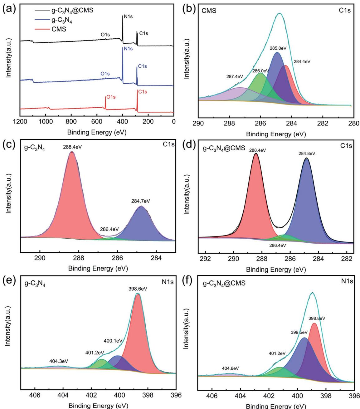
Fig. 2 (a) XPS survey spectrum of CMS,  $g\text{-C}_3\text{N}_4$  and  $g\text{-C}_3\text{N}_4\text{@CMS}$ , (b–d) C 1s high-resolution spectrum of CMS,  $g\text{-C}_3\text{N}_4$  and  $g\text{-C}_3\text{N}_4\text{@CMS}$ , (e, f) N1s high-resolution spectrum of  $g\text{-C}_3\text{N}_4$  and  $g\text{-C}_3\text{N}_4\text{@CMS}$ .
