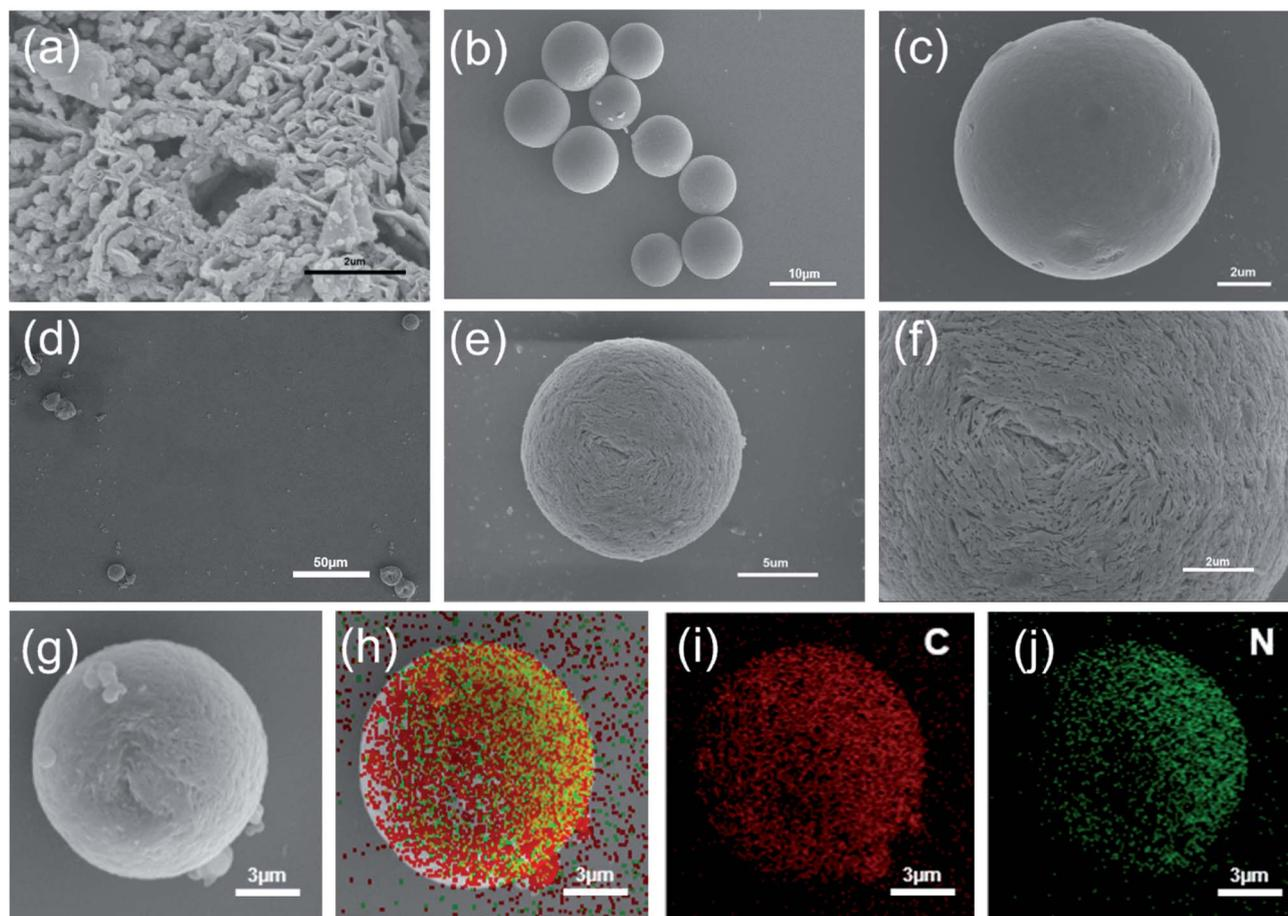
Fig. 1 Micromotor characterization. (a) SEM images of  $g\text{-C}_3\text{N}_4$ , (b) and (c) SEM images of CMS, (d), (e) and (f) SEM images of  $g\text{-C}_3\text{N}_4\text{@CMS}$  micromotor, (g–j)  $g\text{-C}_3\text{N}_4\text{@CMS}$  elemental distributions.
