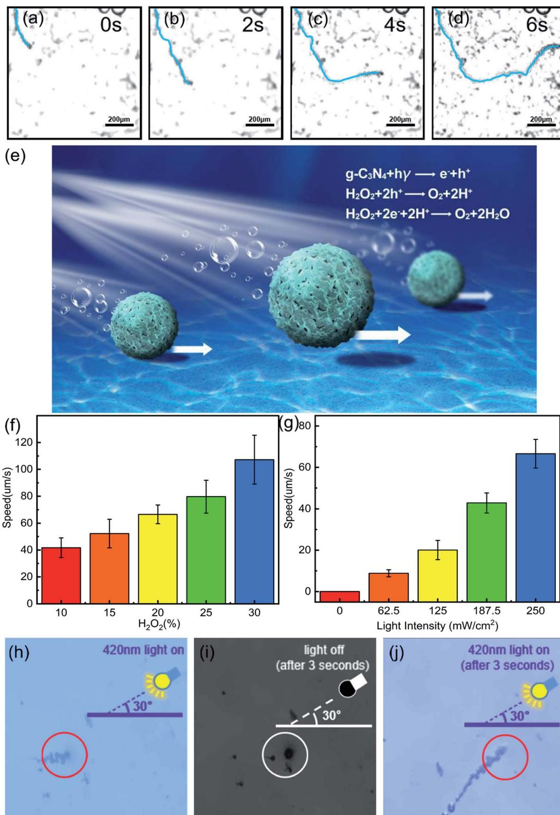
Fig. 5 (a–d)  $g-C_3N_4@CMS$  motion video screenshots at different times (0s, 2s, 4s, 6s) under 420 nm light; (e) schematic representation of the self-propulsion by  $g-C_3N_4@CMS$  micromotors; (f) speed of  $g-C_3N_4@CMS$  micromotor versus  $H_2O_2$  concentration; (g) speed of  $g-C_3N_4@CMS$  micromotor versus light intensity; (h–j) the influence of light on the motion of  $g-C_3N_4@CMS$  micromotor.
