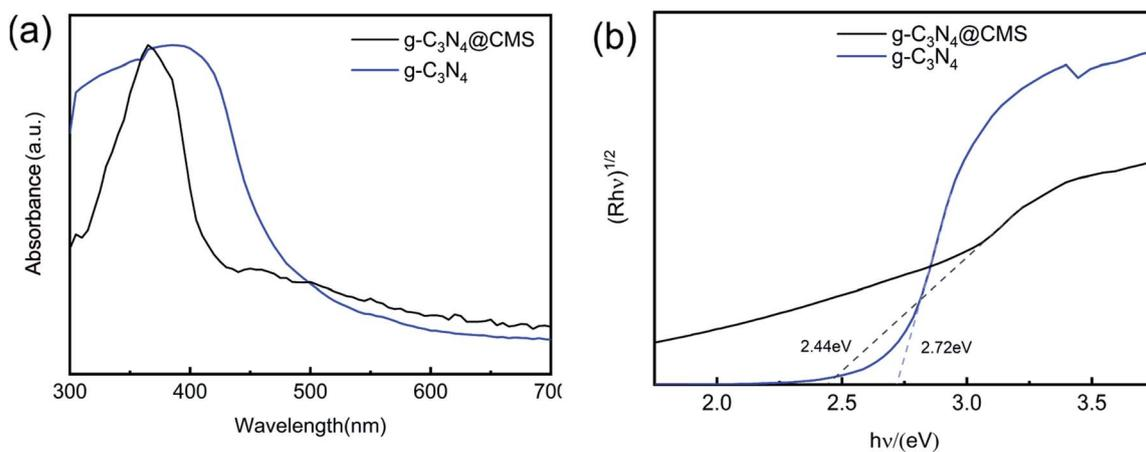
Fig. 4 (a) UV-Vis diffuse absorbance spectra of the g-C<sub>3</sub>N<sub>4</sub> and g-C<sub>3</sub>N<sub>4</sub>@CMS. (b) Plotting of (a) in the  $(\alpha h\nu)^{1/2} \sim$  energy coordinate to evaluate the corresponding bandgap of the g-C<sub>3</sub>N<sub>4</sub> and the g-C<sub>3</sub>N<sub>4</sub>@CMS.
