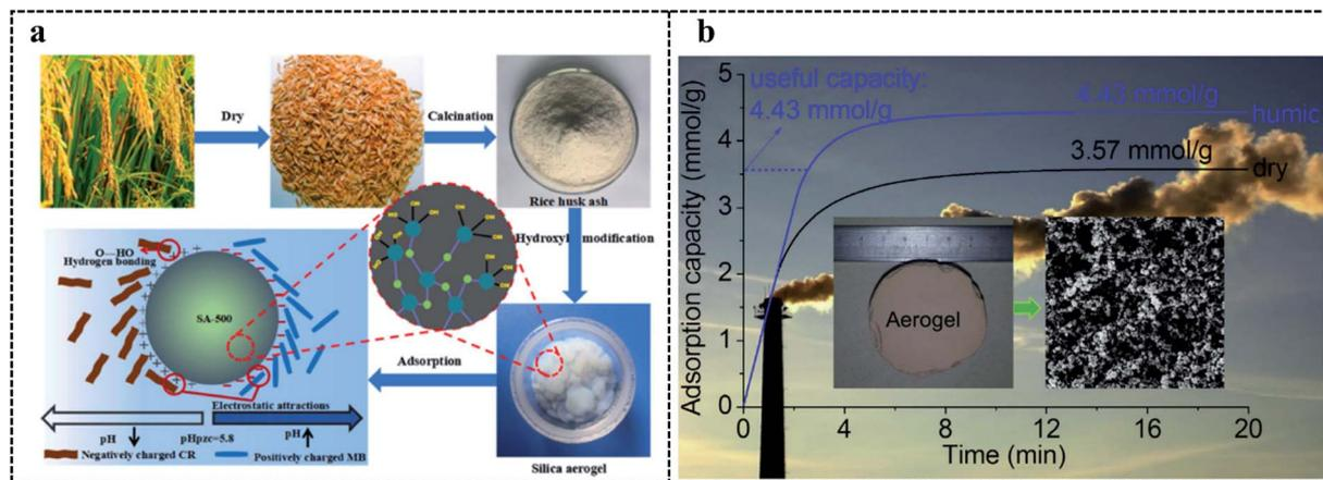
Fig. 6 (a) The adsorption of hydroxyl modified SAs for CR and MB.<sup>187</sup> Copyright 2021, Elsevier. (b) The adsorption of RF/SiO<sub>2</sub> aerogels for CO<sub>2</sub>.<sup>188</sup> Copyright 2015, Elsevier.
