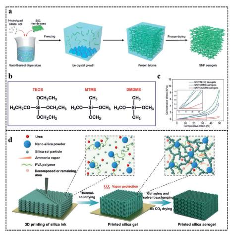
Fig. 4 (a) Synthetic route of SNF aerogels. (b) Structures of different crosslinking silane coupling agents. (c) Compressive  $\sigma$  versus  $\varepsilon$  at the 5th loading–unloading cycle of different SNF aerogels. Copyright 2020, John Wiley and Sons. (d) Synthetic route of thermal-solidifying SAs. Copyright 2021, American Chemical Society.
