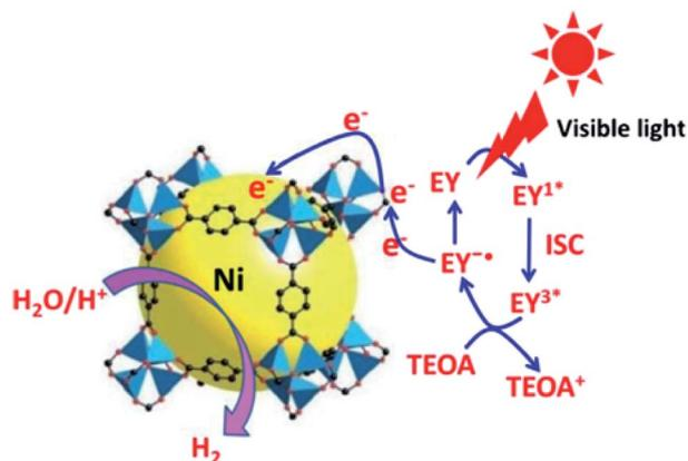
Fig. 8 Photocatalytic pathway for H<sub>2</sub> evolution over the EY sensitized Ni@MOF-5 with TEOA under visible light irradiation, EY = Eosin Y (this figure has been adapted/reproduced from ref. 67 with permission from Elsevier, copyright 2016).
