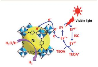
Fig. 8 Photocatalytic pathway for H<sub>2</sub>evolution over the EY sensitisedNi@MOF-5 with TEOA under visible light irradiation, EY = Eosin Y (this figure has been adapted/reproduced from ref. 67 with permission from Elsevier, copyright 2016)
