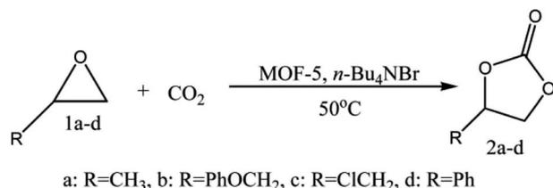
Fig. 3 Coupling of CO<sub>2</sub> with epoxides (this figure has been adapted/reproduced from ref. 41 with permission from Royal Society of Chemistry, copyright 2008).
