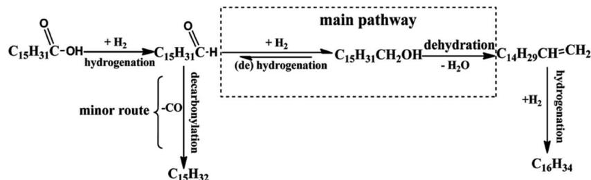
Fig. 6 Proposed hydrogenation process for palmitic acid over PTA@PdCu@Fe<sup>III</sup>-MOF-5 (this figure has been adapted/reproduced from ref. 56 with permission from Royal Society of Chemistry, copyright 2017).
